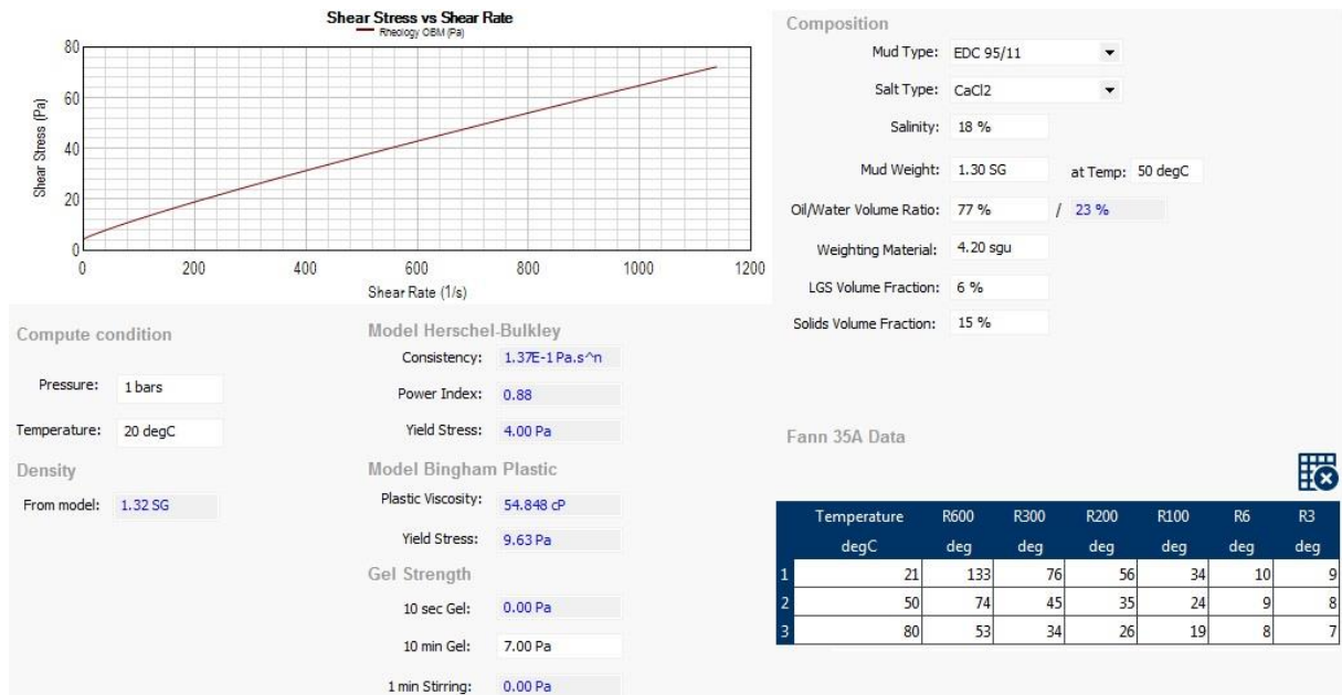
Figure 13: Oil based mud design and rheology[20]
