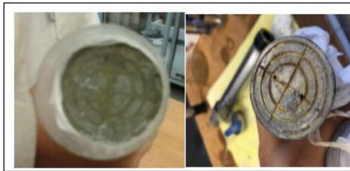
Figure 11 Formation of filter cake during particle injection
