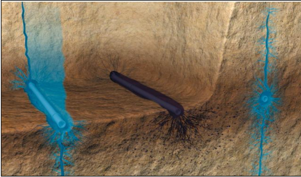
Figure 9: Illustration of FAST technique. Fracture induced in the injector well because of injection pressure (adapted from Rod et al. 2005).
