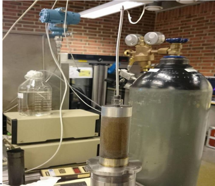
Figure 3.1. Preparation of the core (applying plastic sleeve)
