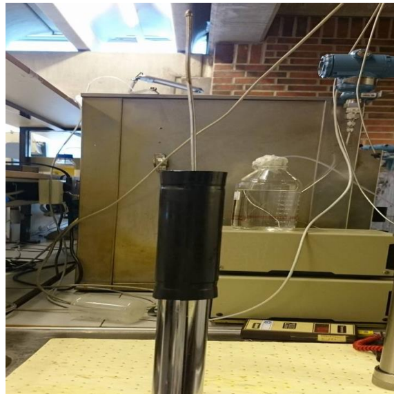
Figure 3.2. Preparation of the core (placing the rubber)
