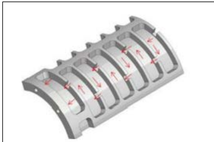
Figure 7: Flow Path through Equalizer Select, (Akbari et al., 2014)
