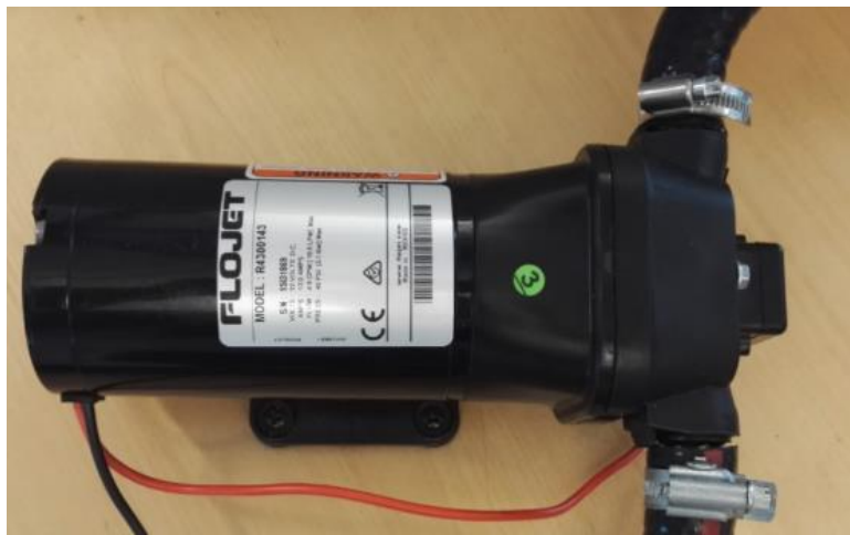
Figure 4.5: Flojet pump, showing the input and outflow connections and electrical cables for the pressure sensor
