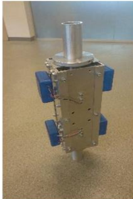
Figure 3.14: Constructed Riser with the load cells
