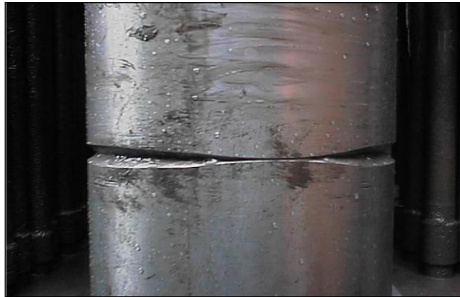
Figure 12: Wear flat that was caused by forward synchronous whirl ( Internal Document - Dynamic Analysis, 2016 )
