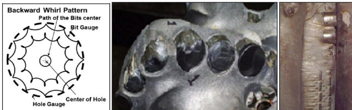
Figure 14: Shoulder cutters of a whirling PDC bit can experience intermittent backward motion. Middle: Chipped or broken cutters due to backward whirl. Right: Rounded blades are also a common consequence ( Internal Document - Dynamic Analysis, 2016 )
