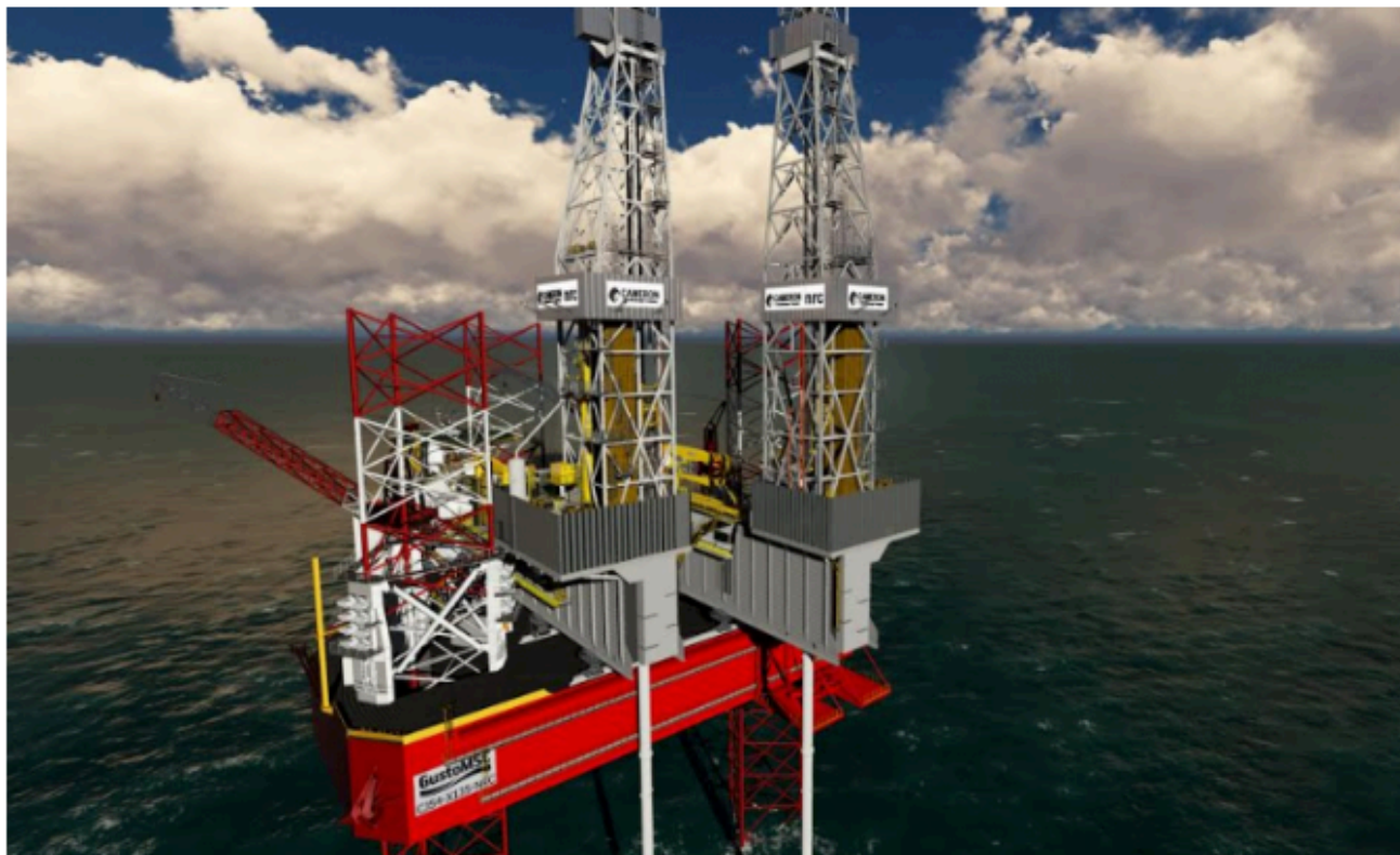
Figure 10: Jack-up especially well-suited for P&A (Stangeland, 2016)
