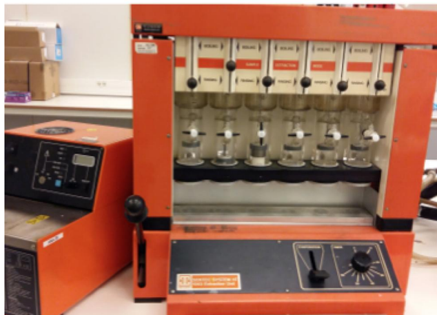
Figure 6.9: Tecator Soxtec System HT 1043 extraction unit (right) and 1046 service unit (left)
