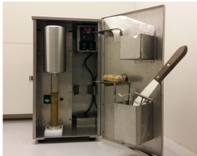
Figure 6.7: Running a retort analysis with OFITE Electronic Retort Kit
