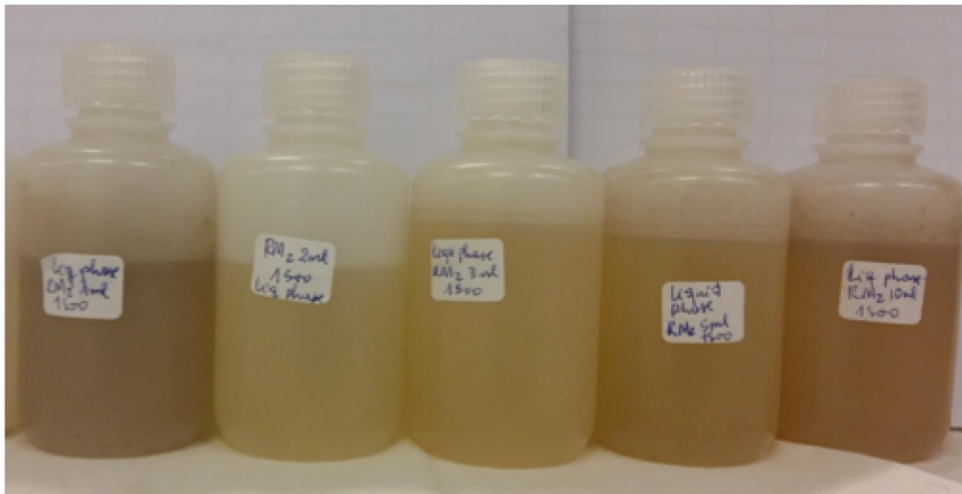
Figure 7.11: Liquid fractions decanted from RM2 samples centrifuged at 435 g versus M2 dosage.
