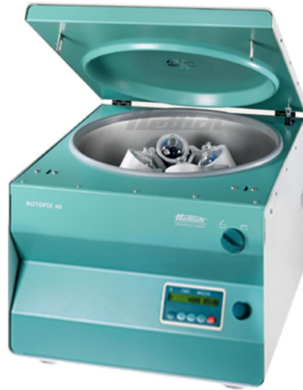
Figure 6.3: Hettich ROTOFIX 46 lab benchtop centrifuge (Hettich Instruments LP)
