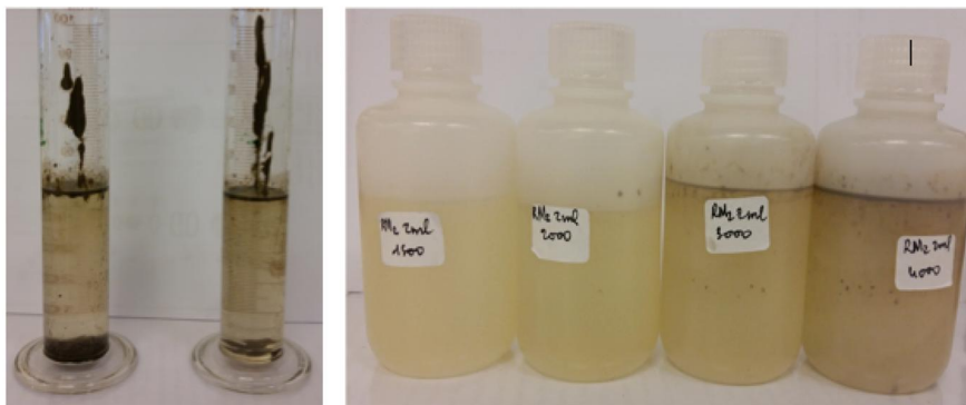
Figure 7.9: Liquid/sludge fraction removed from RM2 samples centrifuged at 3095 g (left) and liquid fraction versus relative centrifugal force (right).
