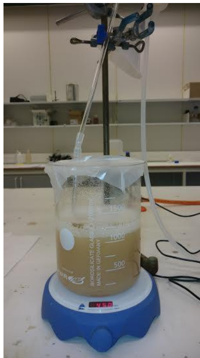
Figure 14: Batch reactor for effluent COD characterization.
