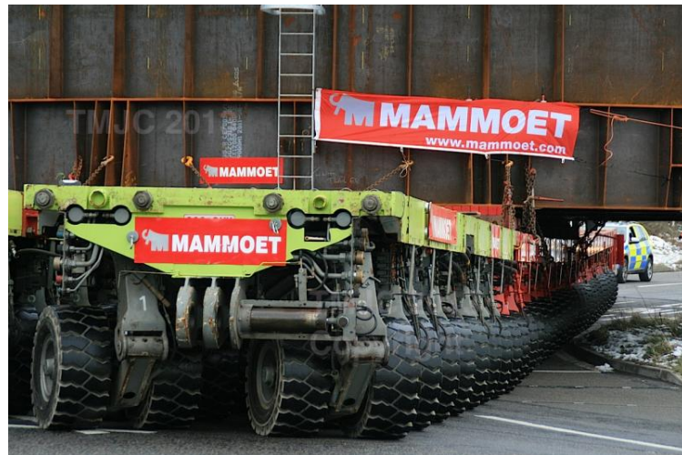
Figure 2-2 Mammoet SPMT's of Belgium. Taken from web link: www.heavyliftspecialist.com
