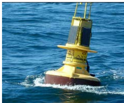
Figure 3-1 AXYS Watkeeper buoy can be deployed in strong currents to collect metocean data. Taken from web link: www.axystechnologies.com
