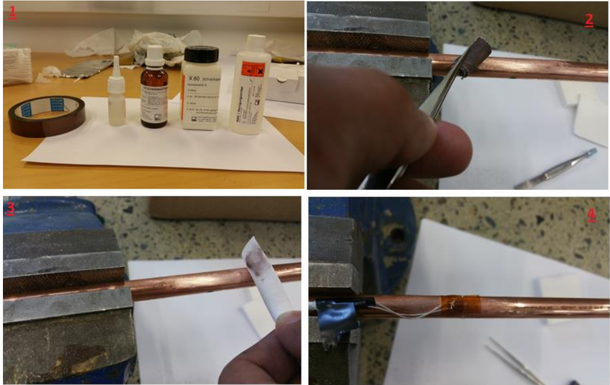
Figure 5-13 Placement of strain gauge. 1 shows the chemical used for strain gauges. 2 Roughing of pipe surface with sand paper. 3 cleaning with acetone and fine cotton paper. 4 placing of strain gauge
