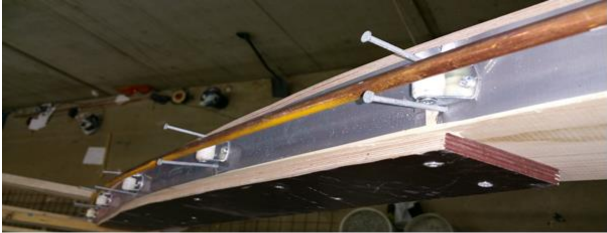
Figure 5-11 Rollers placement on the stinger
