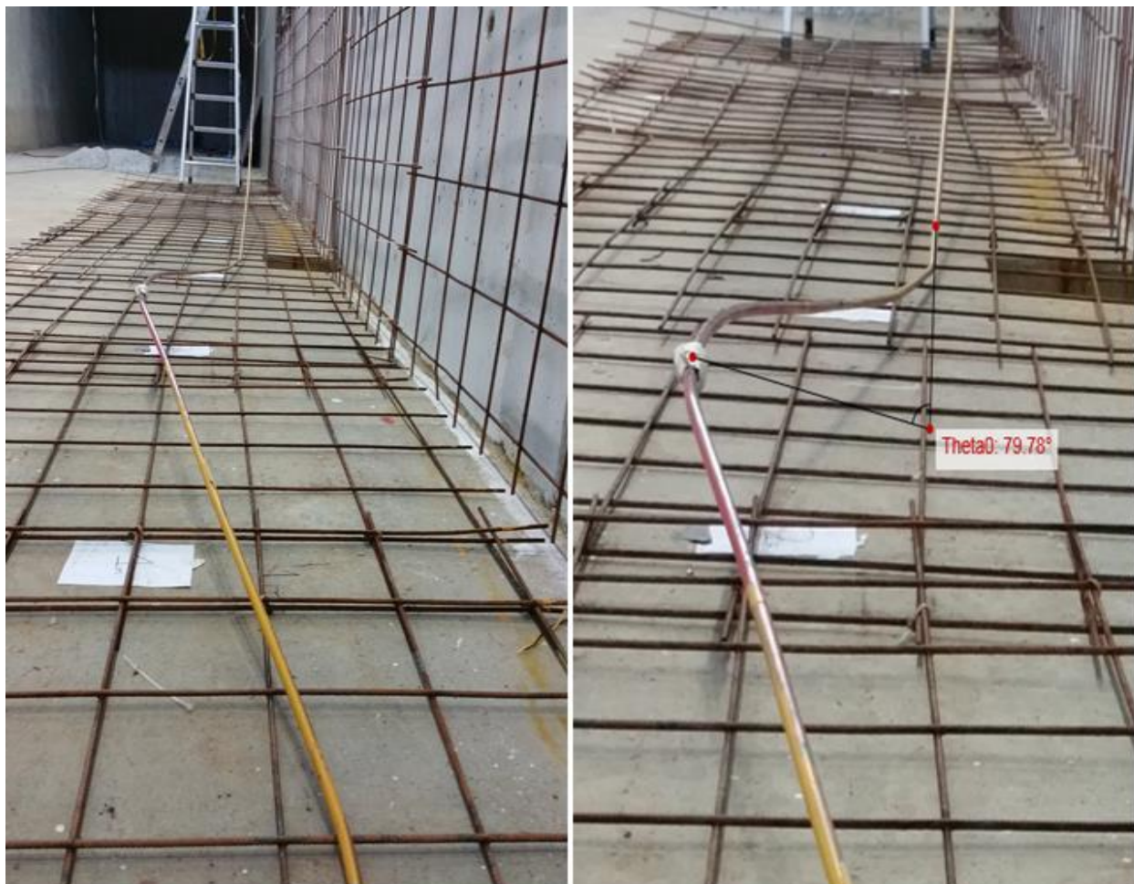
Figure 7-8 Test 1, Pipe at TDP. Right side picture shows the pipe forming the angle with the x-axis obtained by picture digitalization.
