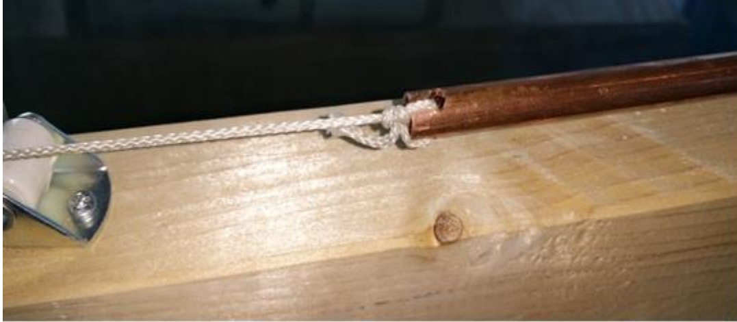
Figure 5-22 Top boundary condition for pipe. Sting is applying the tension force.
