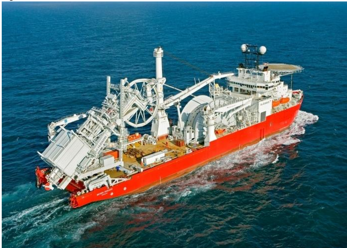
Figure 2-4 Seven Ocean Reeling Vessel, 4-16-inch pipe laying capacity up to 3500 ton of pipe weight, Courtesy of Subsea 7
