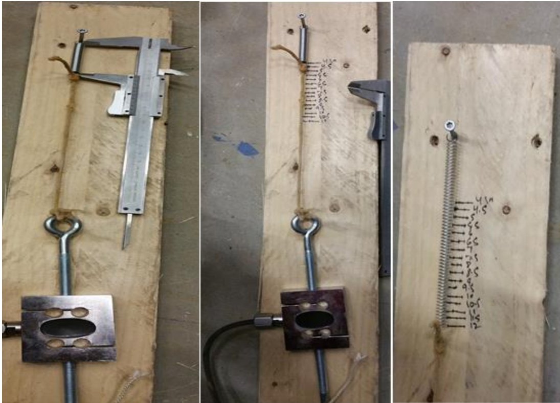
Figure 5-25 Finding spring stiffness by applying force from load cell along known displacements
