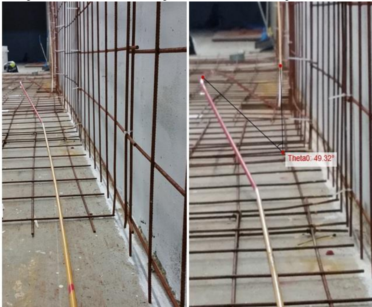
Figure 7-13 Test 14, WD=5.91m, rotation angle at TDP.
