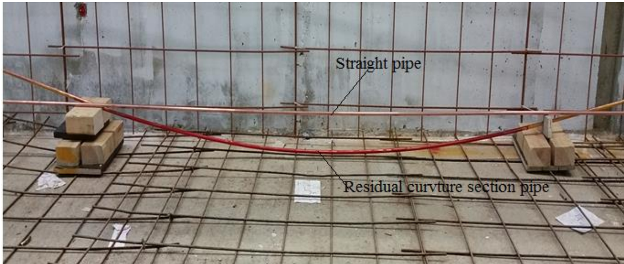
Figure 8-48 Residual curvature section on Uneven seabed
