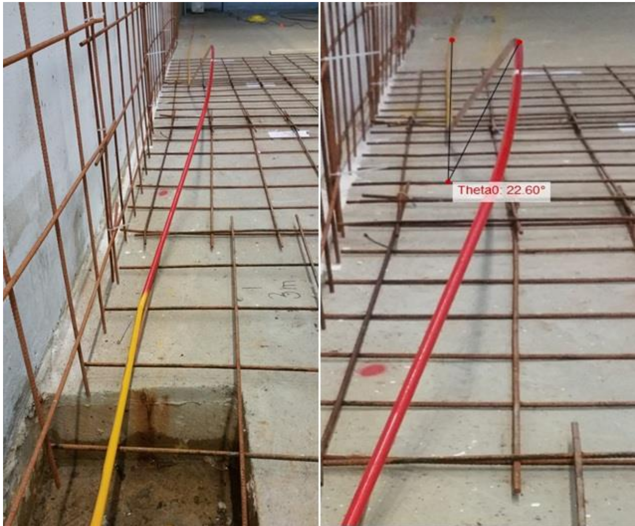
Figure 7-14 Test 16, Fixed Boundary condition, Rotation angle at TDP
