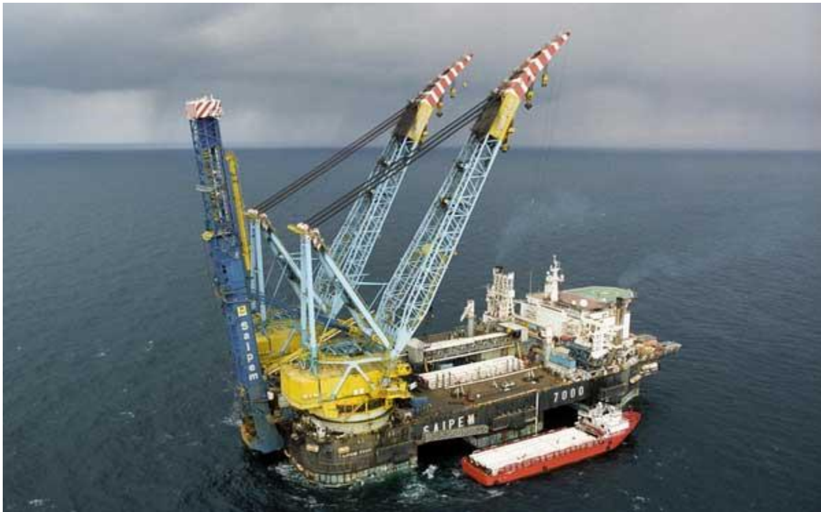
Figure 2-5 a J-Lay semisubmersible vessel for 4"-32" pipe lay, Saipem 7000, Courtesy of Saipem SpA
