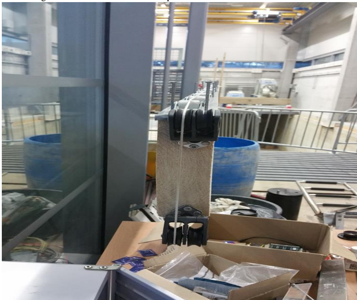
Figure 5-17 Pulley P1 and P2 applying tension through sting at the end of pipe
