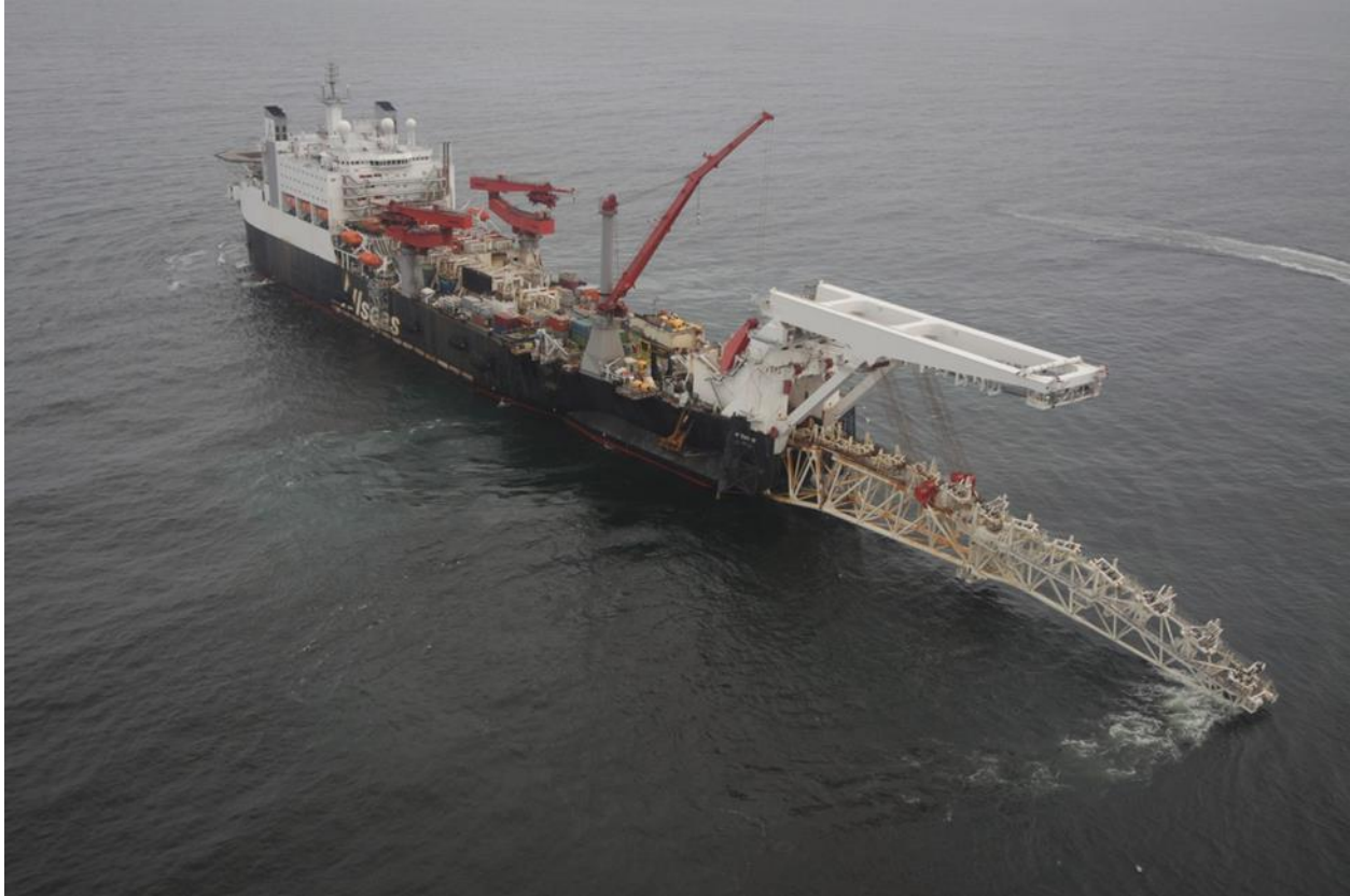
Figure 2-2 S-lay installation vessel Solitaire. 300m long without stinger and has capacity to a holding force of 1050 t. Courtesy of The Allseas Group.
