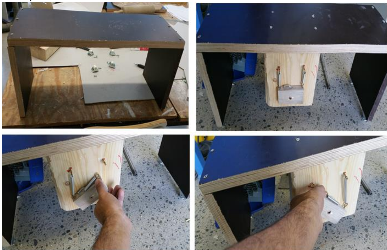
Figure 5-28 Torque measuring device with attached spring
