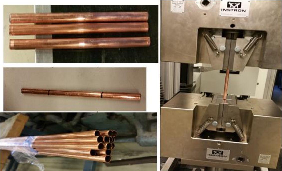
Figure 5-1 three Test samples from the pipes, placed in a tensile testing machine
