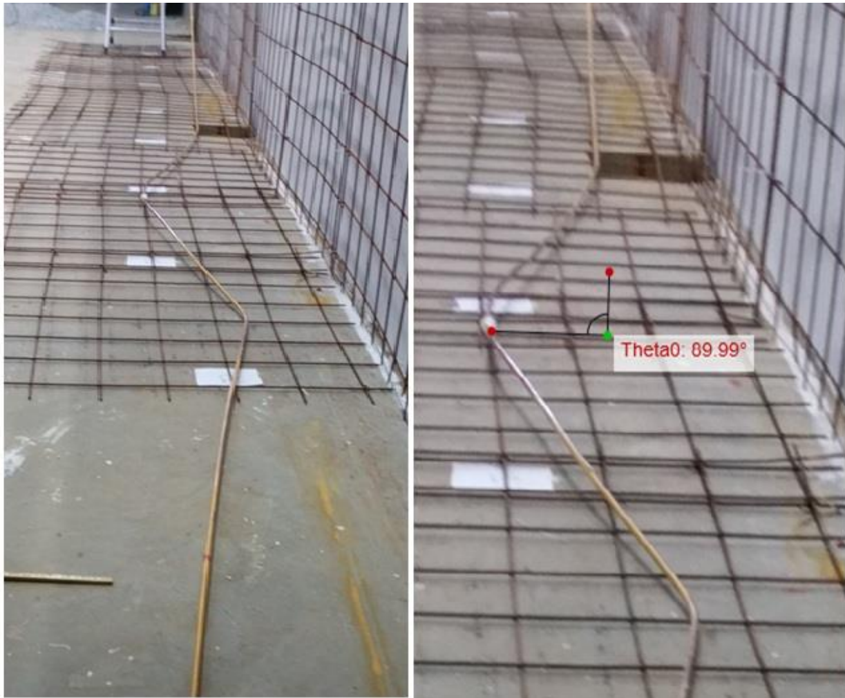
Figure 7-9 Test 2, Pipe at TDP. Right side picture shows the pipe forming the angle with the x-axis obtained by picture digitalization.
