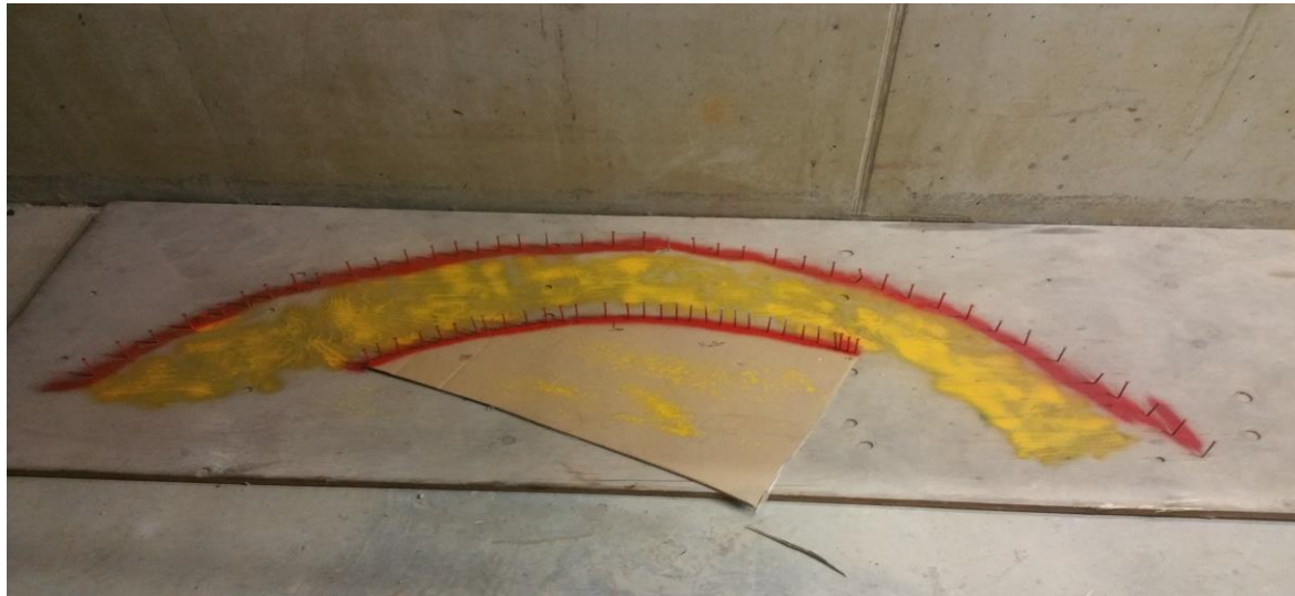
Figure 5-19 Pipe bending set up used to create residual curvature sections
