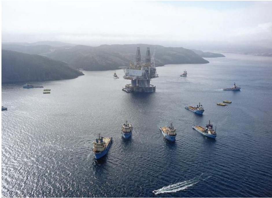
Figure 49. Towing of the Hibernia platform from Bull Arm, Newfoundland, to final location (Photo courtesy of Hibernia Management and Development Company)
