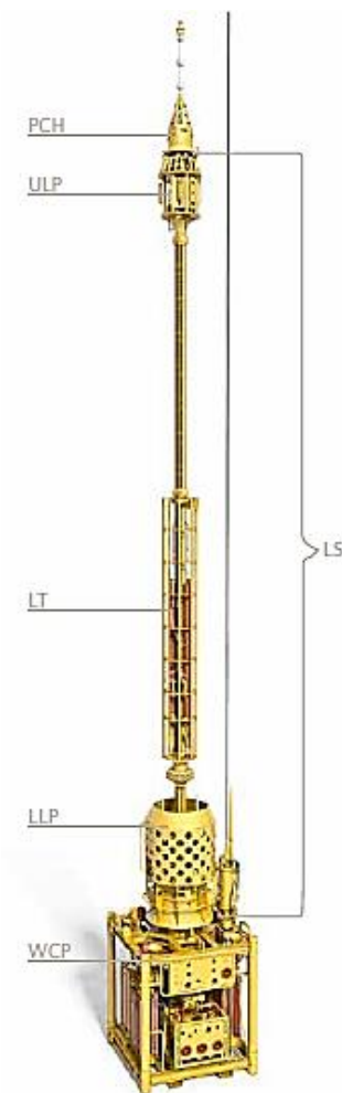
Figure 2-16 FMC RLWI Stack [20]
