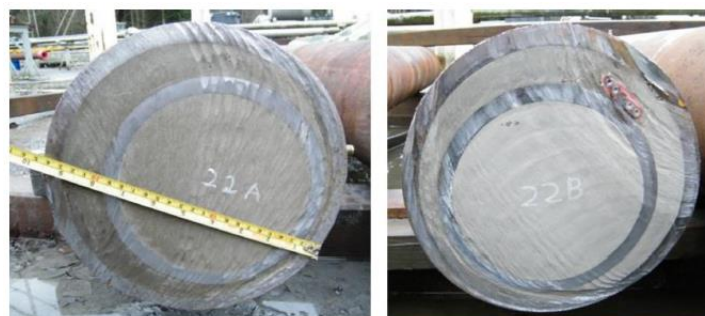
Figure 6-6 Cut Test Assemblies Without Control Lines (left) and With Control Lines (right) [38]
