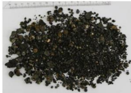
Figure 6-11 Cuttings from Plasma Milling Process [42]
