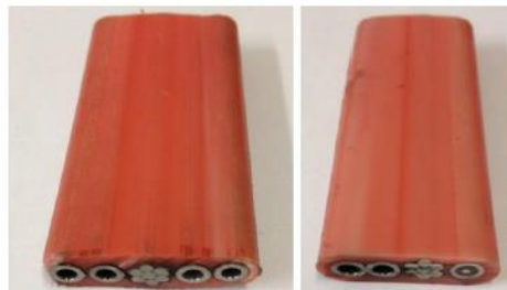
Figure 6-5 Control Cables Used in Tests [38]
