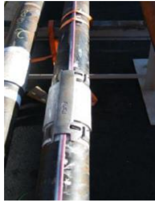
Figure 6-2 Control Lines Outside The Tubing [38]
