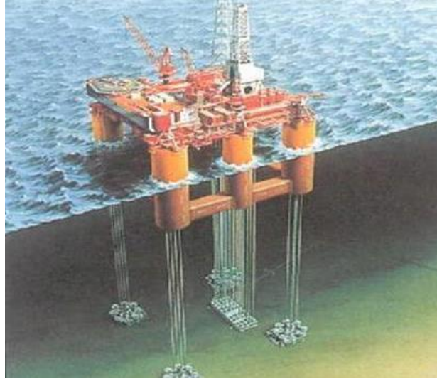
Figure 1-5 conventional Tension Leg Platform (C-TLP) (Paixao, 2016)
