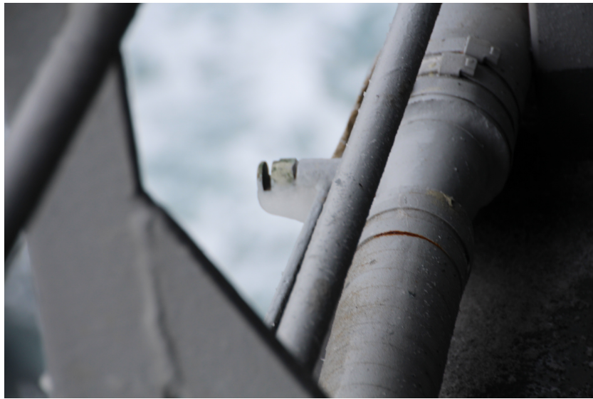
Figure 6.4: Ice accumulation on fire extinguishing nozzle on KV Svalbard. Picture taken in April 2016, west of Ny Ålesund. Ambient temperature was -12^{\circ}\text{C} and no wind apart from the air flow caused by the transit at 13 knots. ©Trond Spande.
