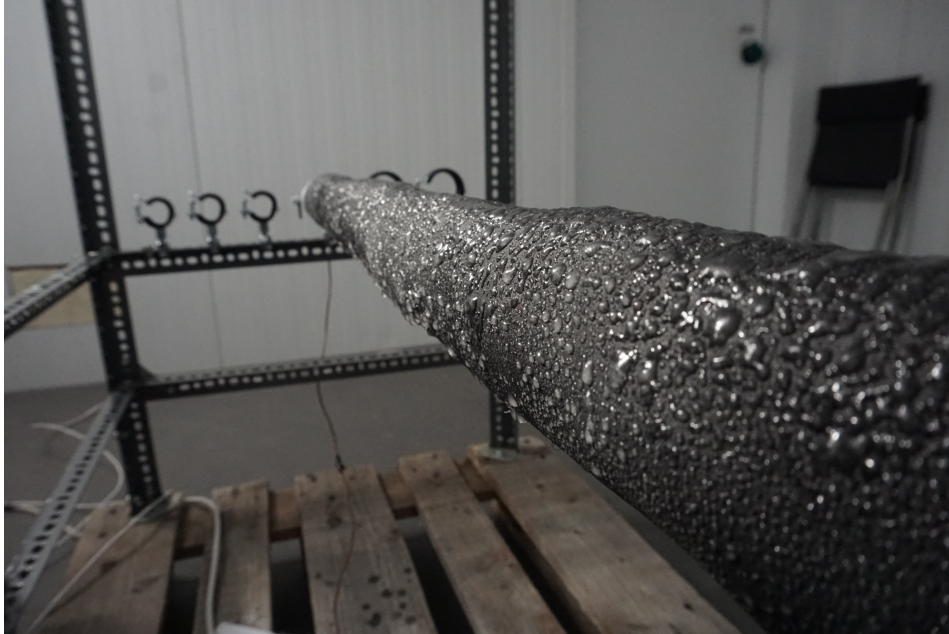
Figure 6.1: Pipe with ice glazing as tested ©Bjarte Odin Kvamme.
