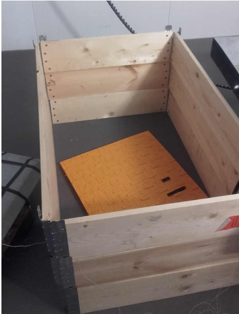
Figure 6.3: Deck element inside pallet boxes to remove any wind from the evaporators. ©Bjarte Odin Kvamme.
