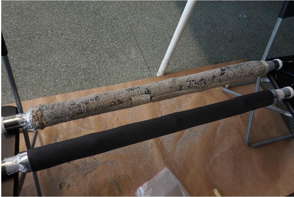
Figure 6.2: Insulated pipe with glued quartz particles versus a normal, insulated pipe ©Bjarte Odin Kvamme.
