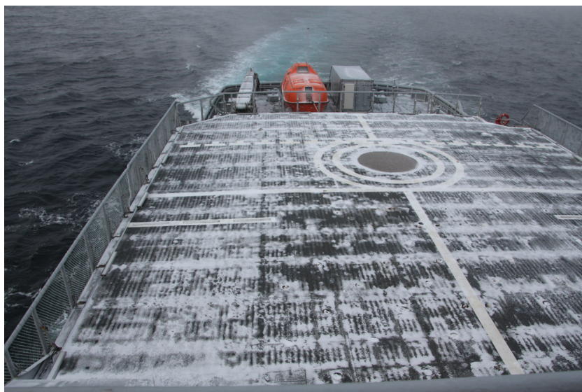
Figure 6.5: Snow and ice accumulation on the helicopter deck on KV Svalbard. Picture taken in April 2016, west of Ny Ålesund. Ambient temperature was -12^{\circ}\text{C} and no wind apart from the air flow caused by the transit at 13 knots. ©Trond Spande.
