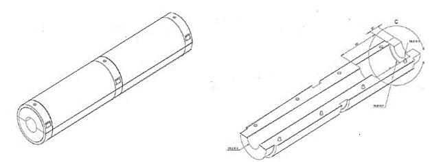
Figure 30 The buoyancy modules as half cylinders with central groove to accommodate the riser (Jhingran et al., 2012).
