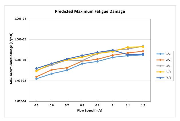
Figure 38 Predicted fatigue damage with default set of parameters (Wu et al., 2016)
