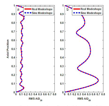
Figure 35 Reconstructed CF displacements for configuration 2-2 at U = 1.0 m/s (Rao et al., 2015)
