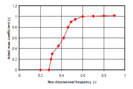
Figure 21 The VIVANA model for added mass as a function of frequency for IL response (Passano et al., 2015)
