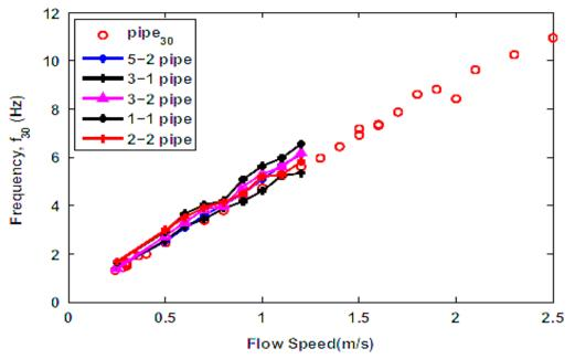
Figure 32 Frequency associated with bare section plotted against flow speed (Rao et al., 2015)
