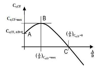
Figure 26 Three point excitation coefficient curve for CF response (Passano et al., 2015)
