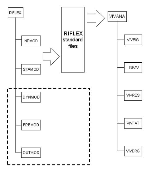
Figure 16 The overall structure of VIVANA (Passano et al., 2015).
