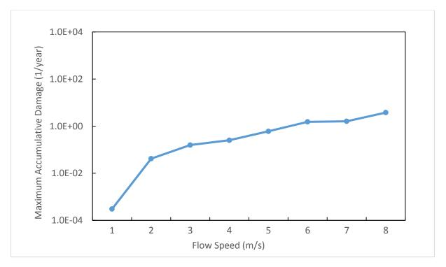
Figure C.1 Maximum accumulated damage for default set of excitation parameters from VIVANA theory manual – bare riser.
