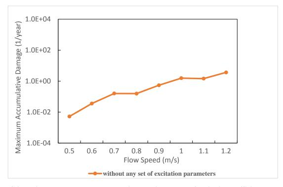
Figure C.3 Maximum accumulated damage without using any set of excitation coefficients – bare riser.
