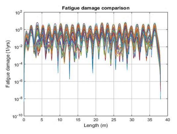
Figure 51 Fatigue damage comparison for different sets of excitation coefficient parameters
