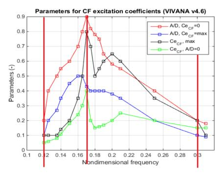
Figure 43 Parameterization of the excitation coefficient curves.
