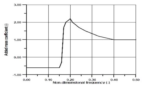
Figure 22 The VIVANA model for added mass as a function of frequency for CF VIV (Passano et al., 2015)
