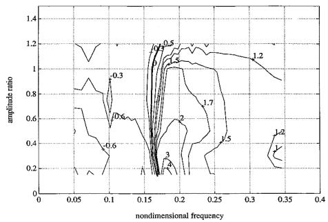
Figure 14 Contours of the CF added mass coefficient (Gopalkrishnan, 1993).
