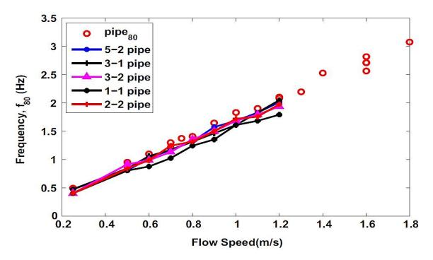
Figure 33 Frequency associated with buoyancy section against flow speed (Rao et al., 2015)
