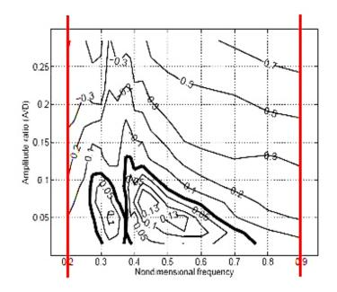
Figure 23 Contour plot curves for the IL excitation coefficient (Gopalkrishnan, 1993).
