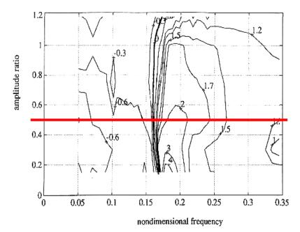
Figure 19 Contour plot of the CF added mass coefficients based on forced harmonic motions (Gopalkrishnan, 1993)
