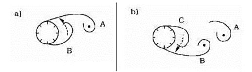
Figure 7 (a): Prior to shedding of Vortex A, B is being drawn across the wake. (b): Prior to shedding B, Vortex C is being drawn across the wake (Sumer & Fredsøe, 2006)
