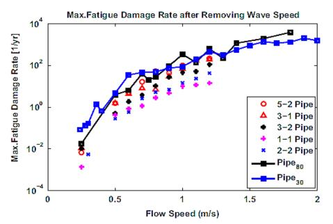
Figure 34 Max. fatigue damage rate plotted against flow velocity (Rao et al., 2015)
