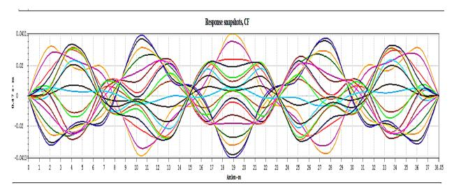
Figure 40 Snapshots of CF displacement with default set of parameters for 2-2 configuration at 1.0 m/s (Wu et al., 2016)
