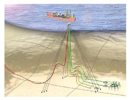
Figure 1 A schematic of SLWR (Jhingran et al., 2012)
