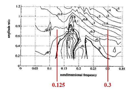
Figure 24 Contour plot curves for CF excitation coefficient (Gopalkrishnan, 1993)
