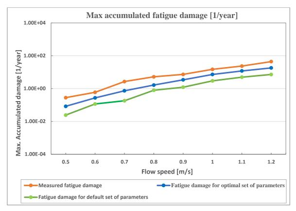
Figure 56 Comparison between measured fatigue damage, fatigue damage for optimal set of parameters and for default set of parameters.
