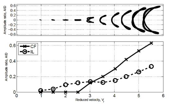
Figure 9 The lower figure shows maximum response amplitude in IL and CF direction, while the upper figure shows the corresponding response trajectory at mid-span (Aronsen, 2007).
