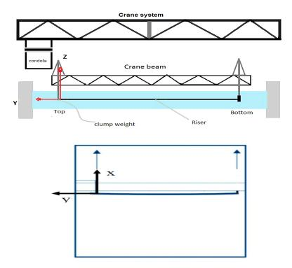
Figure 28 Test setup and coordinate system; upper: front view; lower: top view (Jhingran et al., 2012).
