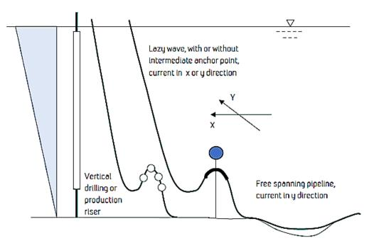
Figure 15 Examples of slender structures that can be analysed by VIVANA (Passano et al., 2015)
