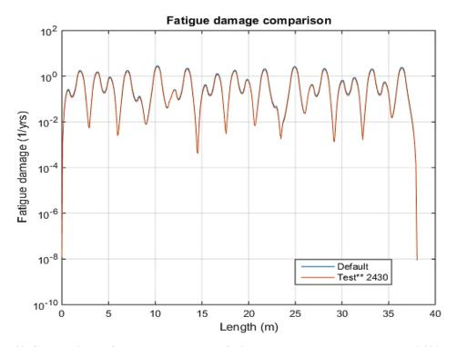
Figure 49 Comparison of max. accumulated fatigue damage between Test no. 2430 and default case.
