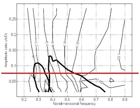
Figure 20 Contour plot of the CF added mass coefficients based on forced harmonic motions (Passano et al., 2015)
