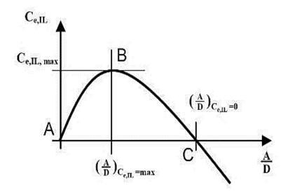
Figure 25 Three point excitation coefficient curve for pure IL response (Passano et al., 2015)
