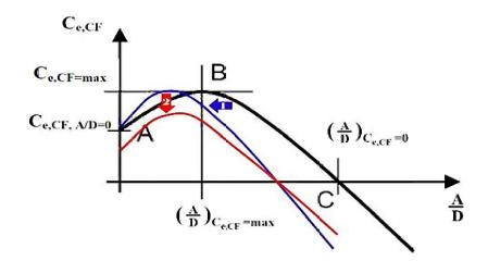
Figure 42 Black curve: default CF excitation coefficient curve at particular non-dimensional frequency in VIVANA, Blue curve: after amplitude modification, red curve: after excitation coefficient modification (Yin et al., 2015).
