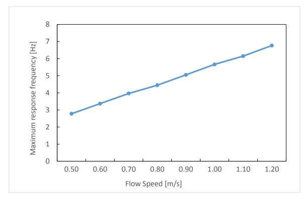
Figure C.2 Response frequency for default set of excitation coefficients from VIVANA theory manual – bare riser.
