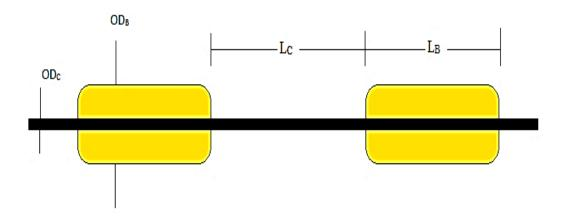
Figure 29 Definition of gap lengths and buoyancy segment lengths (Jhingran et al., 2012)
