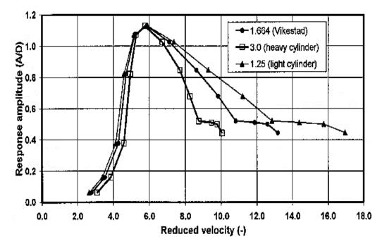
Figure 12 Response amplitudes for three cylinders with different weights (Larsen, 2011)
