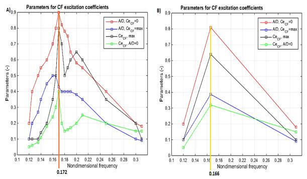
Figure 47 Comparision between the contour curves of A) default set of parameters and B) set of parameters for Test no. 2197.
