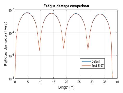
Figure 46 Comparison of accumulated fatigue damage between Test no. 2197 and default case.
