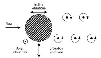
Figure 8 Motion of cylinder due to vortex shedding (Le Cunff et al., 2002)
