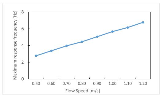
Figure C.4 Maximum response frequency without using any set of excitation parameters– bare riser.
