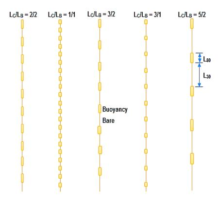
Figure 31 Staggered buoyancy configurations over the riser (Rao et al., 2015)
