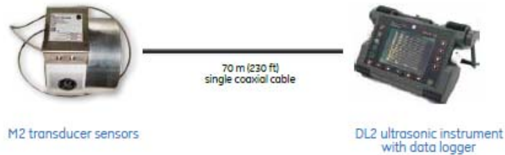
Figure 5.4: Portable Low Temperature (LT) Installed Manual System
