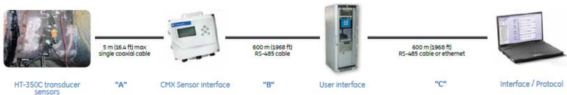
Figure 5.6: Portable High Temperature (LT) Installed Automated System
