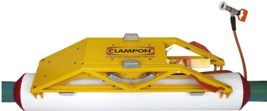
Figure 5.17: Clamp-On CEM Real time/ Offline Corrosion-Erosion Monitoring System Operating Principle of Clamp-On CEM:
