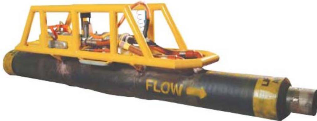
Figure 4.13: Field Signature Method Technology CorrOcean
