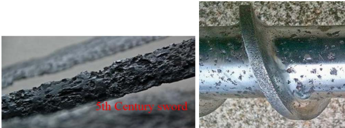
Figure 4.6: Pitting Corrosion due to scratches, impurities
