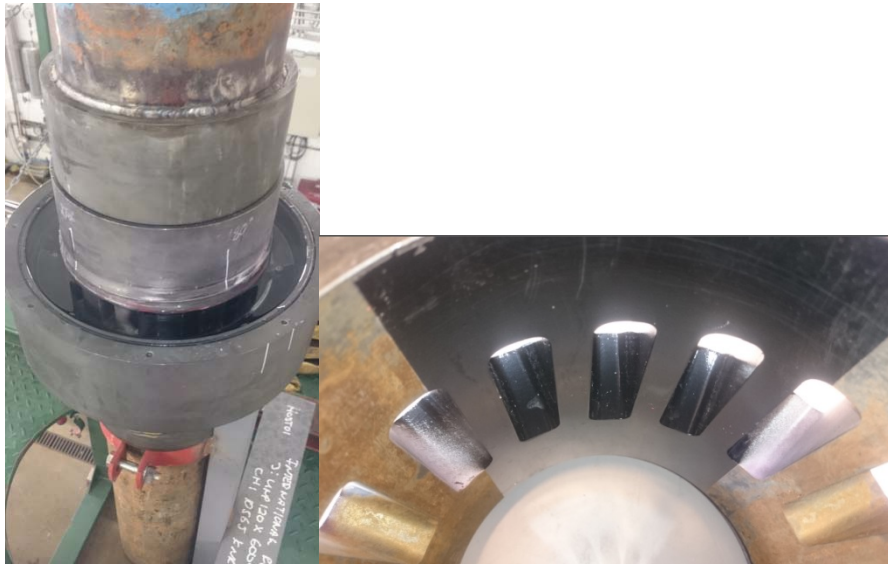
Figures 3.2 : Sand Slurry Test Set Up & Unpainted Rusted Inner Sleeve Slots
