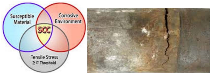
Figure 4.9: Stress Corrosion Cracking
