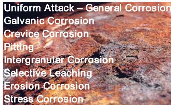
Figure 4.2: Basic Types of Corrosion common in OG Industry
