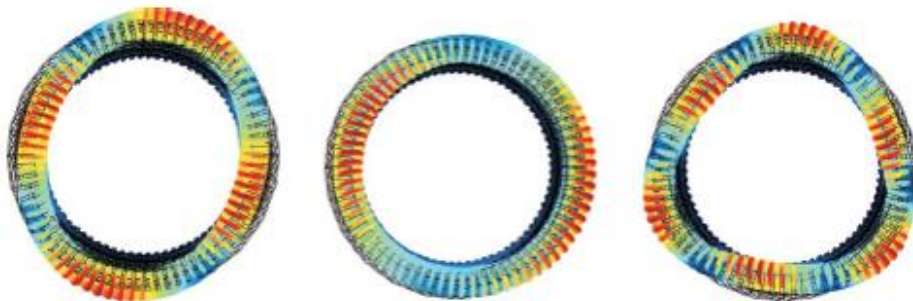
Figure 16: Stator endwinding deformation due to electromagnetic forces. Image source: JIP project.
