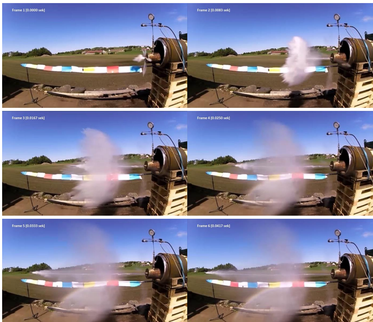
Figure 17 Captions of projectile discharge during test
