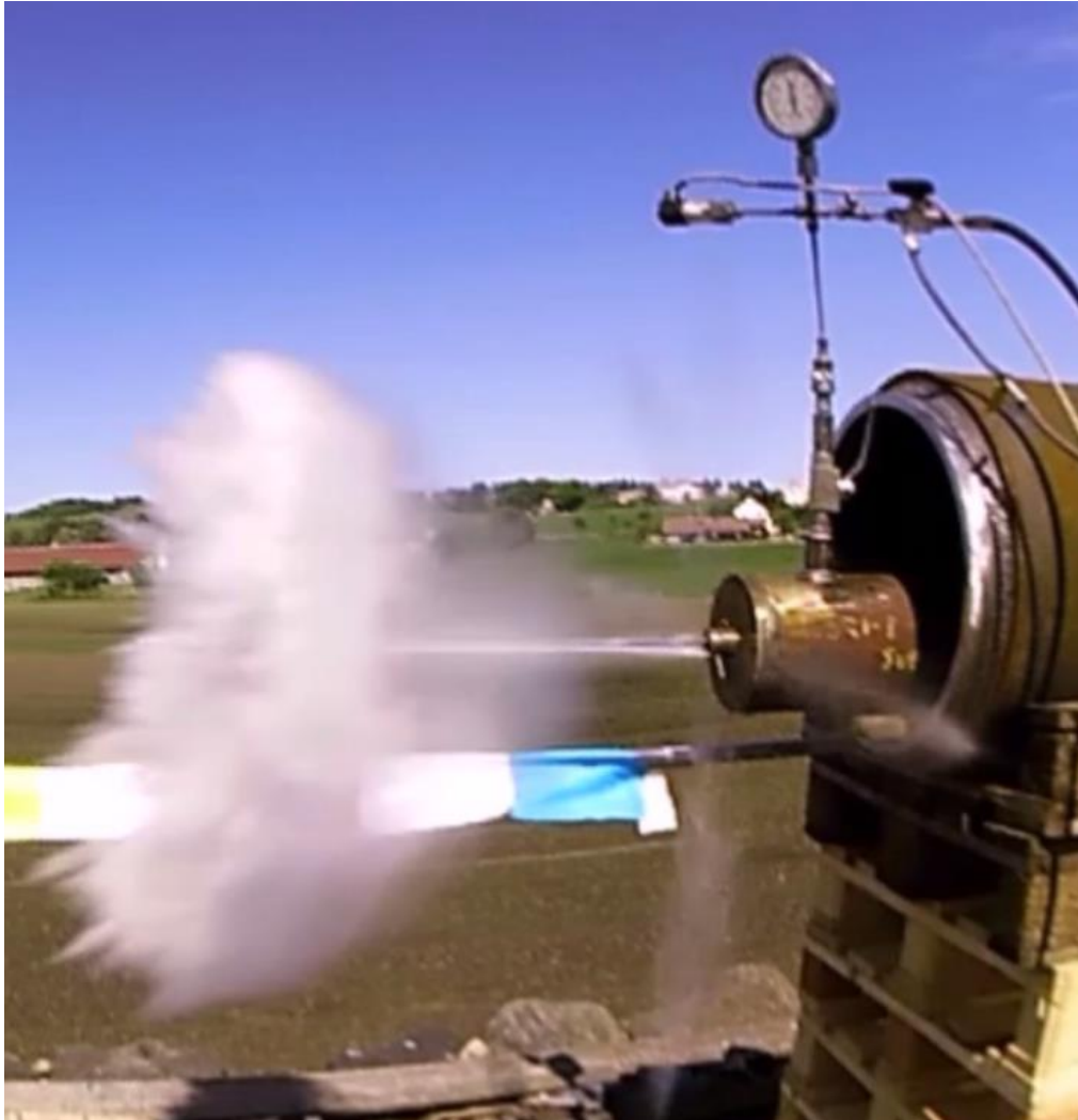
Figure 7 Water jet during projectile test
