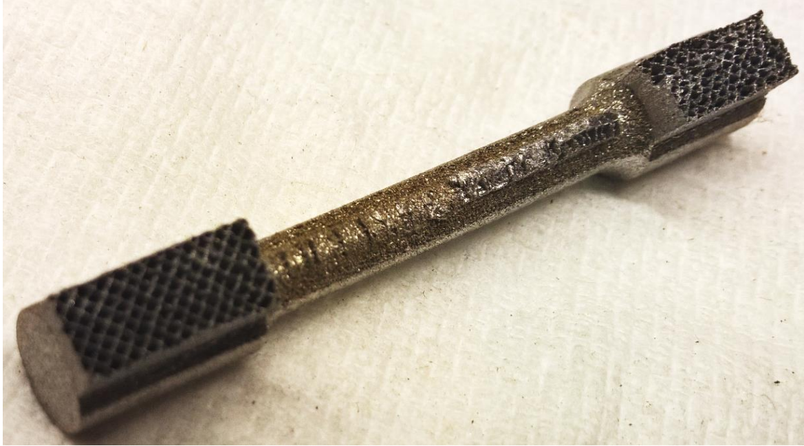
Figure 4.1.2-1 Rough overhang and support structure on specimen L1
