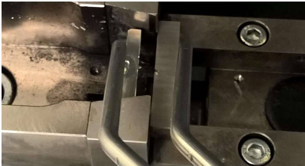
Figure 3.3.3-1 Specimen being placed in the testing machine with a self-centring tong. The wedge in the tong centres the specimen in the correct position relative to the wedge on the pendulum.
