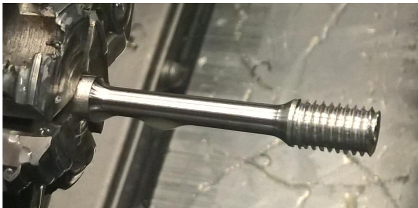
Figure 3.2.2-2 U-specimen after “SS5M8P2.MIN”. The profile has been cut and one end threaded.
