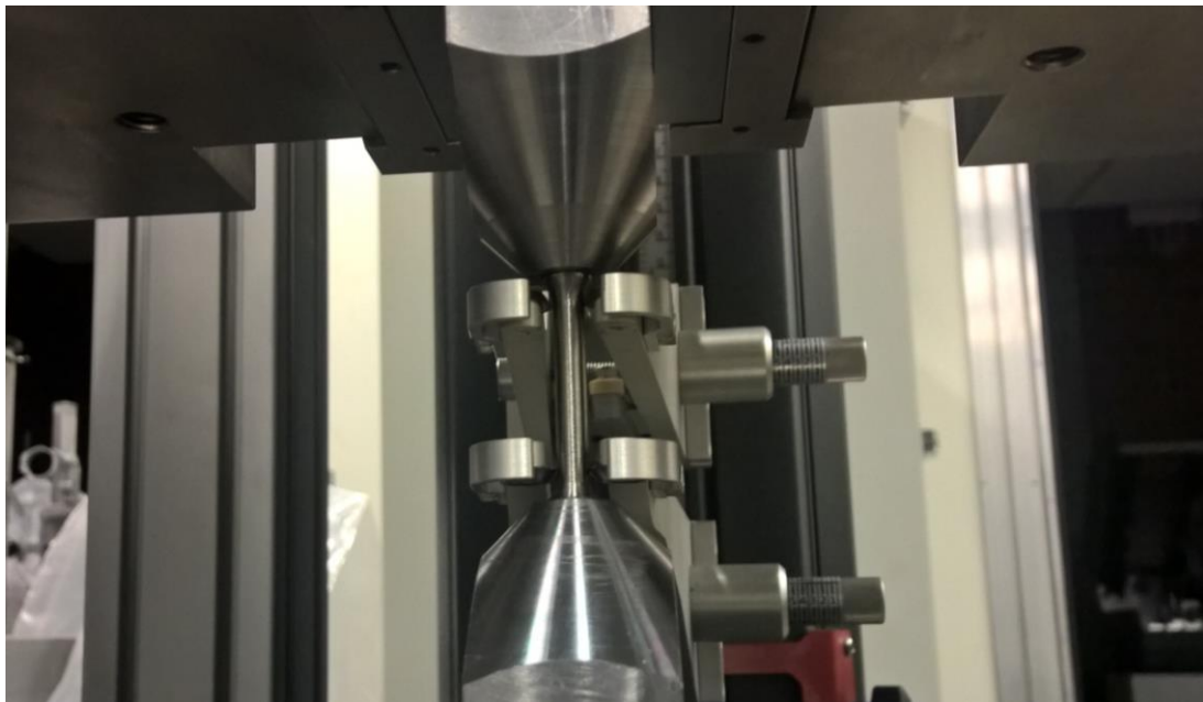
Figure 3.2.3-1 Specimen U1 mounted and ready for testing. Extensometer in place and specimen fastened in mounts.
