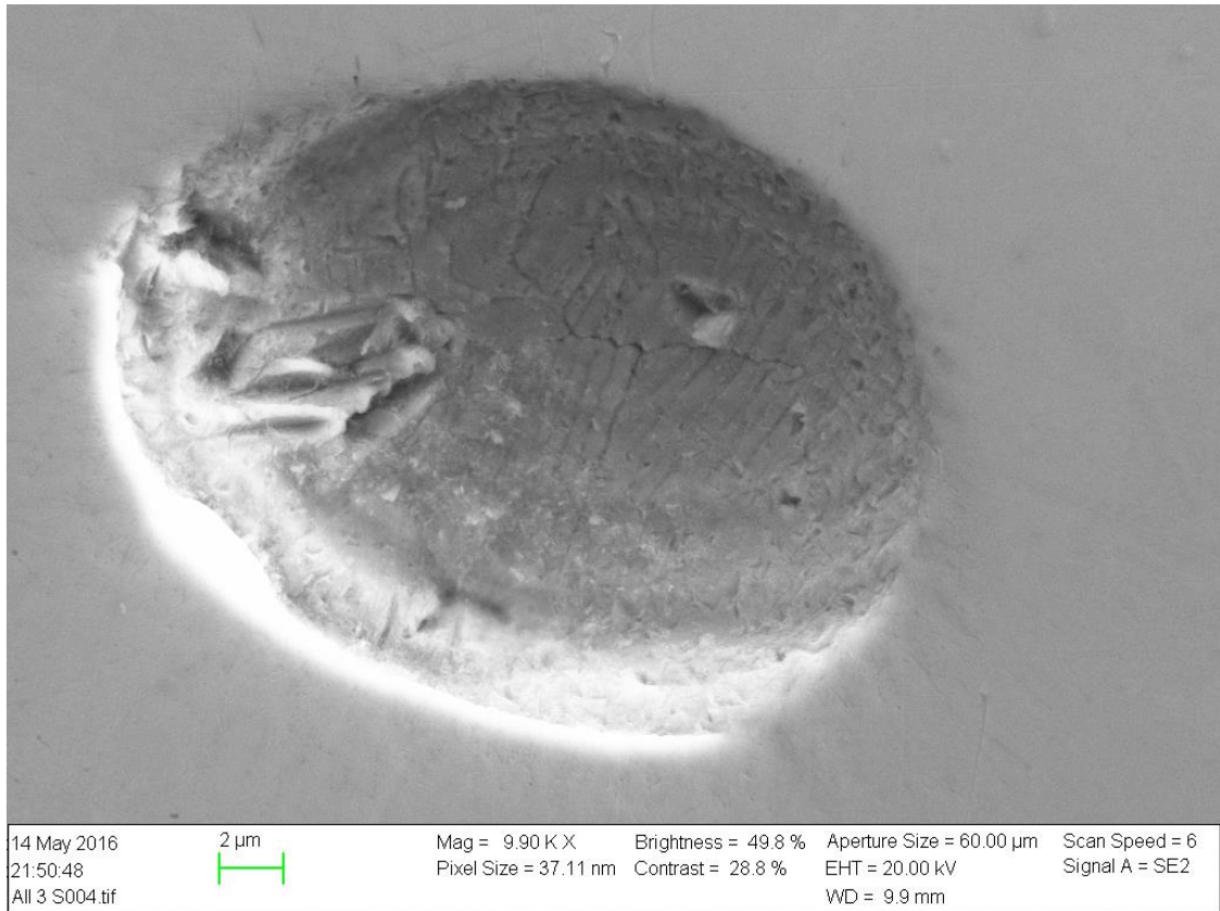
Figure 4.7.1-2 Pore in surface of A II 3 S up close. Cracks visible at the bottom.
