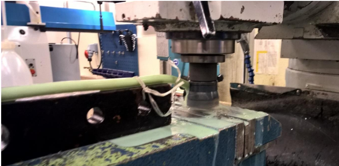
Figure 3.3.2-1 Face milling off support structure on CharpyV-specimen.
