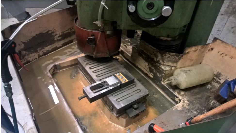
Figure 3.3.2-3 Grinding setup for a Charpy specimen
