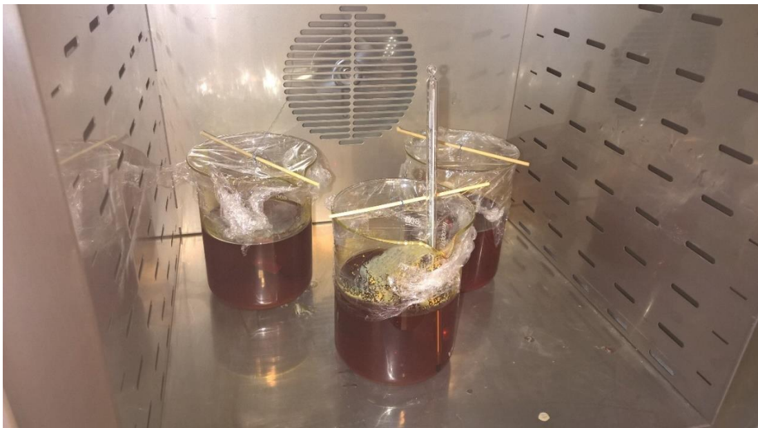
Figure 3.5.3-1 Corrosion tests in the heating cabinet after 24hours. Test 1, 2, and 3 from left to right with the thermometer in the middle.
