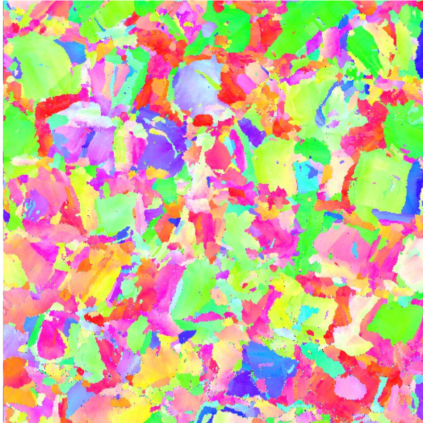
Figure 4.7.4-2 Grain orientation, specimen seen from the top and down, xy-plane. 500x500 \mu\text{m} .
