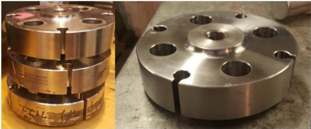
Figure 22: Before and after picture of flanges after cleaning and machining
