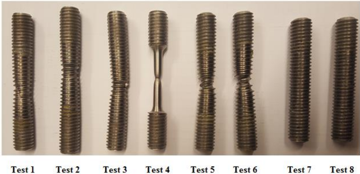
Figure 30: Bolts after tensile testing
