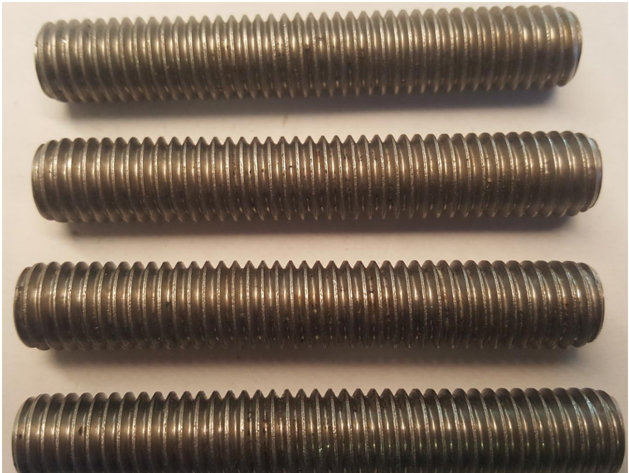
Figure 37: 316L bolts from alternate immersion testing after cleaning
