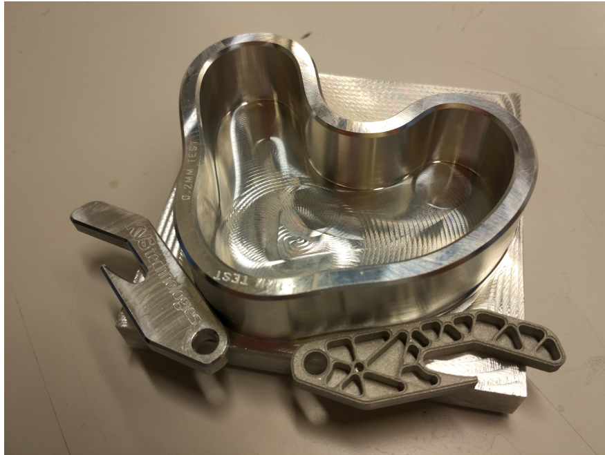
Figure 2: Traditionally machined parts made out of aluminium 6082-T6 in a Mazak 430A Vertical Mill at the University of Stavanger
