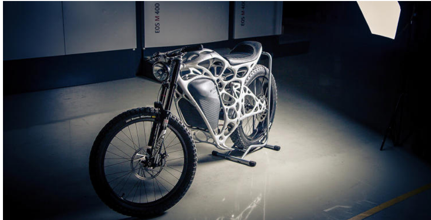
Figure 24: Topology optimized skeleton frame motorcycle, by airbus APWORKS[18]
