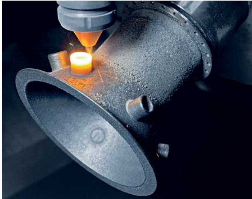
Figure 7: Directed energy deposition method for manufacturing an object[8]
