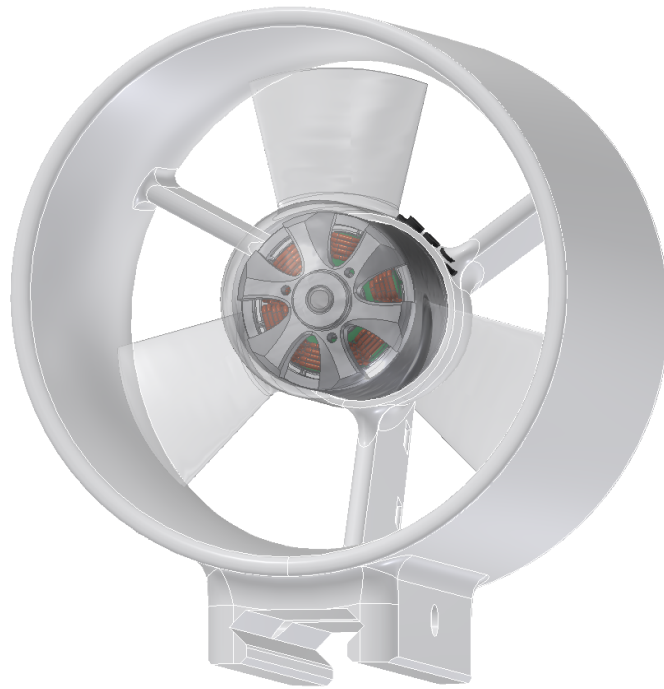
Figure 14: An overview of part I: thruster housing, shown with transparent propeller(Part II) and DC outrunner motor.
