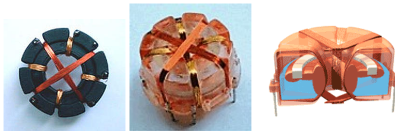
Figur 3.2: Fluxgatesensor fra Autonnic Research Limited
