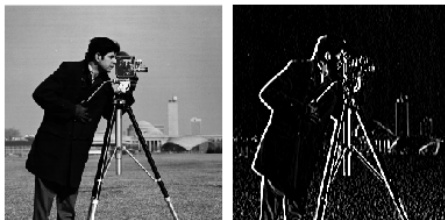
Figure 2.16: A test image convolved with the Sobel vertical edge detector.
