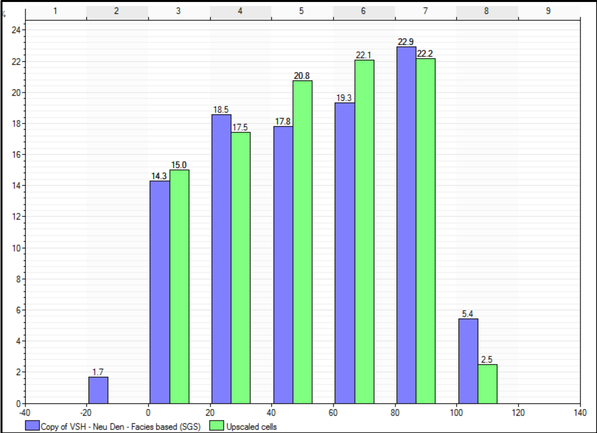
Figure 63: Histogram displaying the differences in the percentage of Vsh distributed across the model from the up-scaled well logs and the property model.
