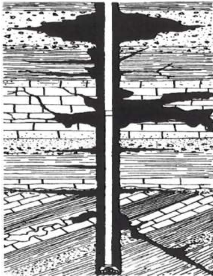
Figure 2.1: Types of loss circulation formations [15].
