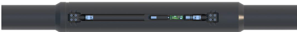
Figure 20 Downhole memory gauge[18]
