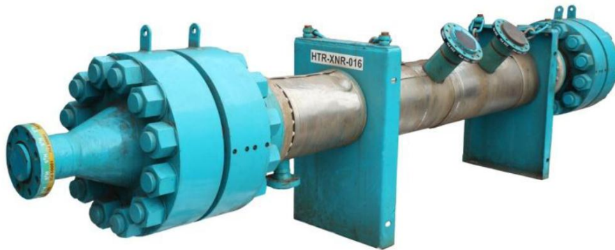
Figure 13 Multitube Heat Exchanger
