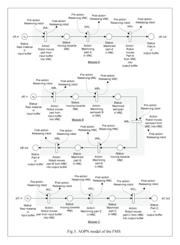
General propose Petri Net Simulator (GPenSIM) is a realization of AOPN methodology that is available for MATLAB platform [5]. GPenSIM provides the resource management so that a modeler following AOPN methodology needs only to concentrate of how the jobs (consisting of many activities) can be modeled individually, one at a time, and then combined together to make the complete model.
