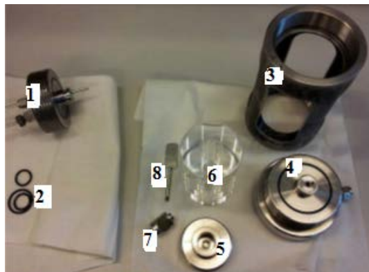
Figure 10. Components of the 23mL sapphire cell. 1 is the top lid with pressure and temperature sensors, 2 are the O-ring ceilings, 3 is protective cap, 4 is connection between bottom lid and sapphire cell, 5 is bottom lid, 6 is sapphire tube (cell), 7 is magnet holder, 8 is stirrer blade.
