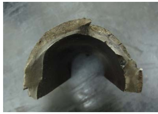
(a) Fatigue fracture of drill collar thread (b) Fatigue fracture of drill pipe body
