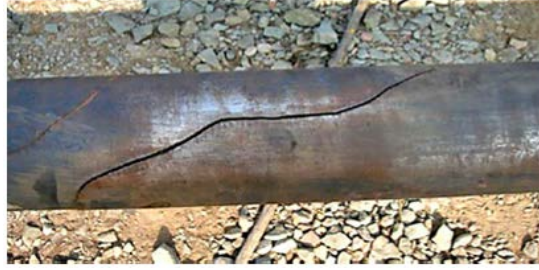
Figure 3-4 Hydrogen sulfide stress corrosion cracking of drill pipe (SSC)
