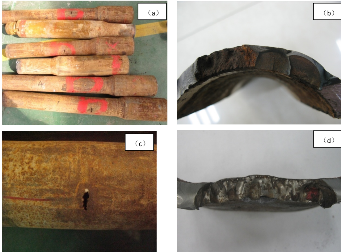
(a) Puncture macroscopic morphology (b) Fatigue crack extend from inner wall (c) Puncture macroscopic of pipe body (d) Crack extend from out wall to inner wall
