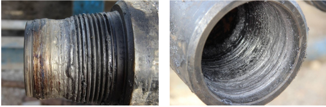
Figure 3-8 Thread gluing due to improper fastening
