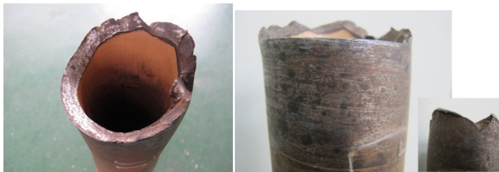
Figure 3-2 Fracture failure morphology due to over twist and overload
