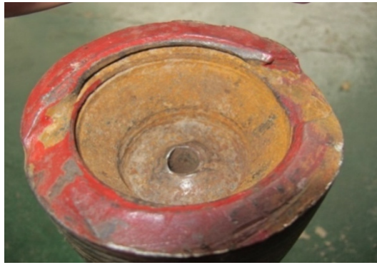
(a) Fatigue fracture of drill collar thread (b) Fatigue fracture of drill pipe body
