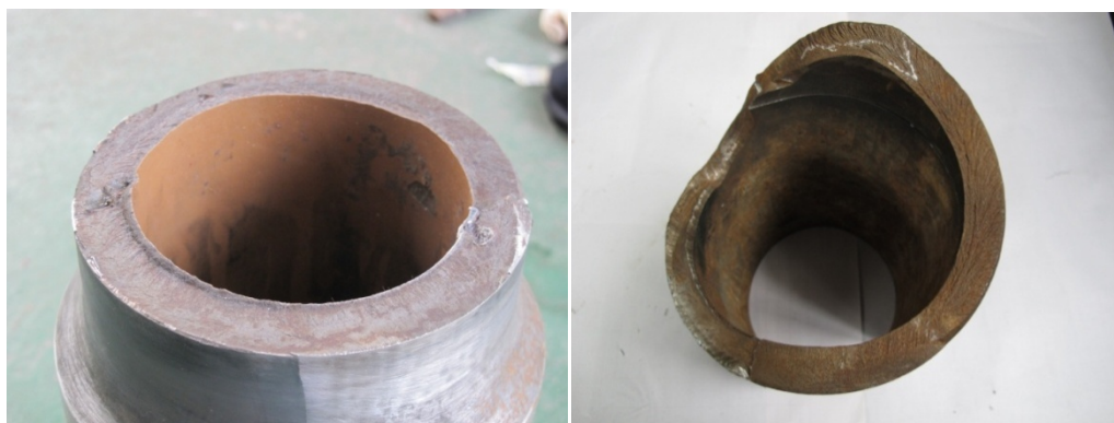
Figure 3-3 Morphology of low stress brittle fracture
