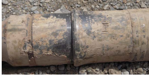
Figure 3-9 Thread joint expansion of female joint
