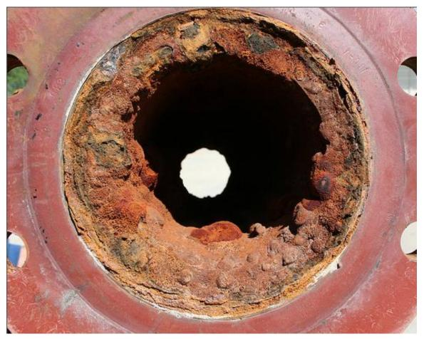
Figure 2.12: Internal CO2 corrosion. (Liberty corrosion, n.d)
