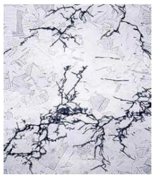
Figure 2.15: SCC in a 316 stainless steel chemical processing pipe. (NACE international, n.d.)
