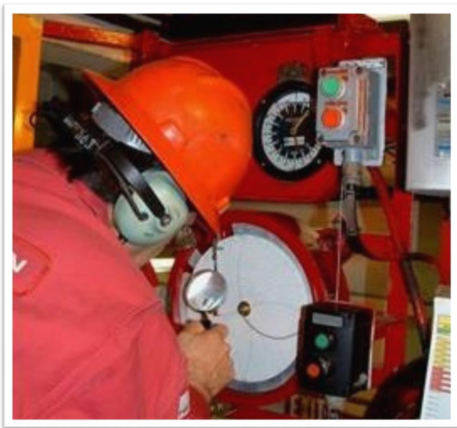
Figure 10: Traditional circular chart for pressure test recording
