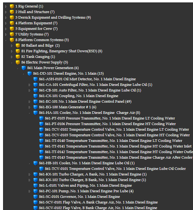
Figure 14 - Technical Hierarchy – Main engine, adapted from KAMFER
