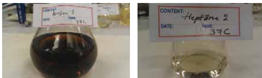
Figure 2. A sample of the kerosene effluent colored by the presence of crude oil in core 37C (left) and a clear heptane effluent after completing the kerosene injection in core 37C (right).
