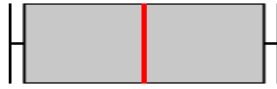
Figure 4.6: Example of a box plot. The horizontal lines on the left and right side represent the min and max values. The grey box is defined by the fifth and ninety fifth percentile values, and the red horizontal line represents the median. It is easy to see that the values are relatively evenly distributed and the median, is in the middle of the figure. This example was generated from the values min: 1495540962 max: 1495541000 mean: 1495540981 median: 1495540981 variance: 240.6667 5th percentile: 1495540964 95th percentile: 1495540998.
