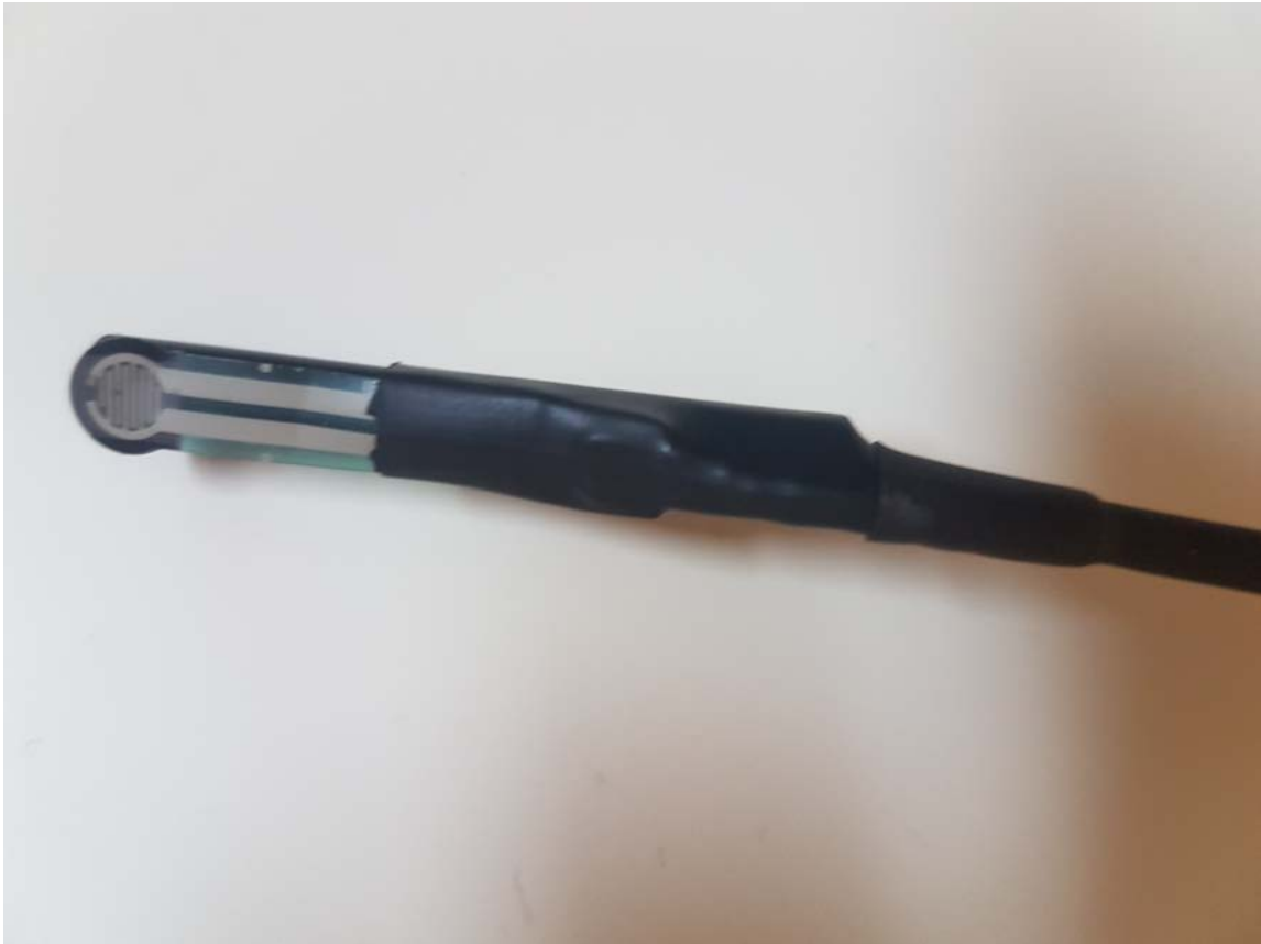
Figure 4: Force Sensitive Resistor taped to a plastic piece
