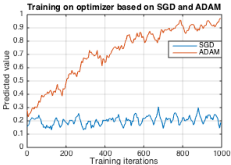
Figure 2.18: Training network with SGD (in blue) vs ADAM (in orange). This is a rather extreme scenario, the SGD struggles to find improvement, given enough time SGD should reach ADAM's prediction.
