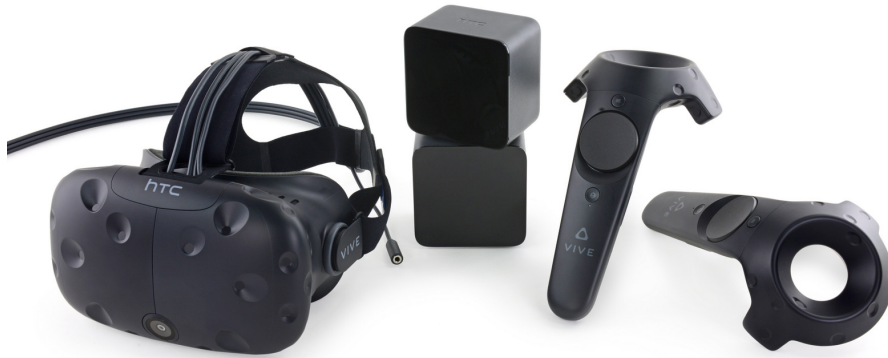
Figure 2.1: The content of a HTC Vive setup; the Head Mounted Device, two hand controllers, and two Lighthouses.[4]
