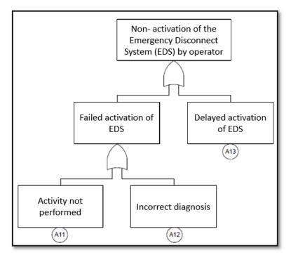
Figure 14 Fault tree of operator barrier element failure (Sklet et al., 2005)
