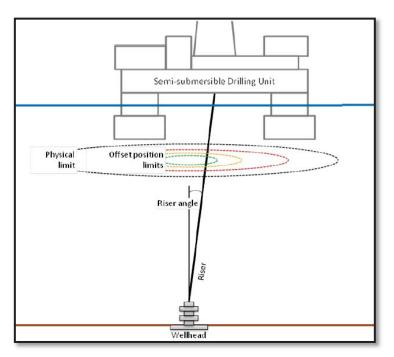
Figure 20 Dynamic positioning drilling operation (Bye et al., 2017)
