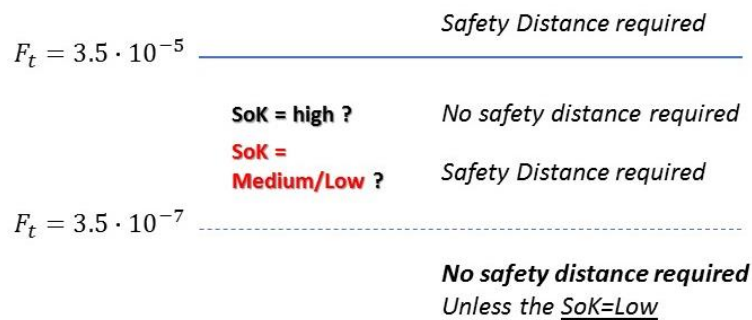
Figure 6.2. Safety distance determination in relation to the SoK the harm frequencies are based on, aligned to the approach on RAC suggested by Aven, 2014.
