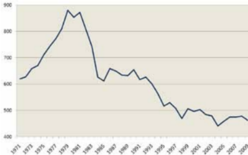
Figure 4.3: The water consumption presented as number of liters per person per 24 hours. The specific consumption has been relatively stable for the last decade (Stavanger kommune, 2010a).
