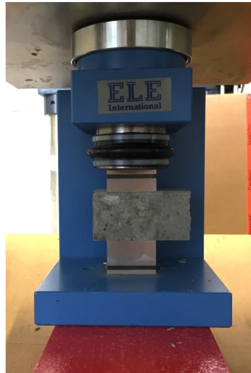
Figure 59. Test setup - Compressive Strength Test (Kjaernsmo, 2017)
