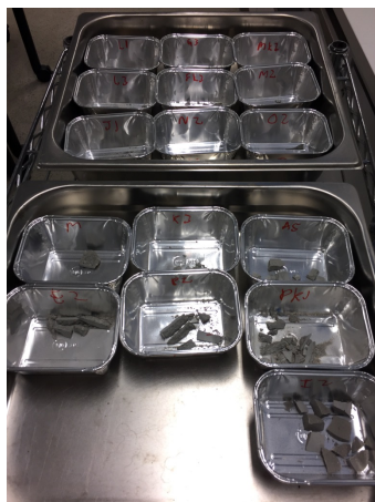
Figure 69. Small samples were taken from central parts from the fractured surface (Kjaernsmo, 2017)
