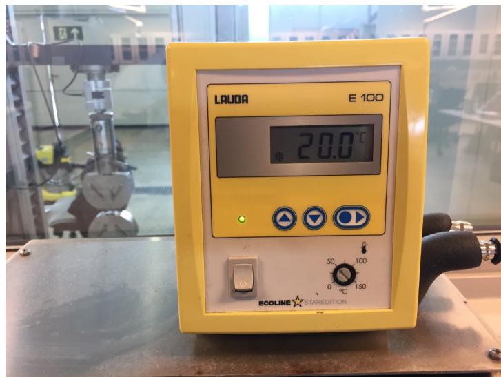
Figure 39. Lauda Temperature Control Unit & Circulator (Kjaernsmo, 2017)
