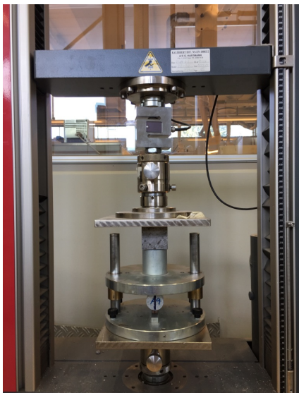
Figure 60. Test Setup - Splitting Tension Strength Test
