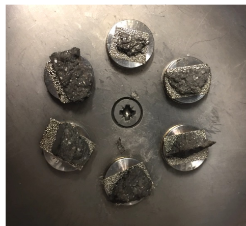
Figure 72. The samples with palladium cover (Kjaernsmo, 2017)
