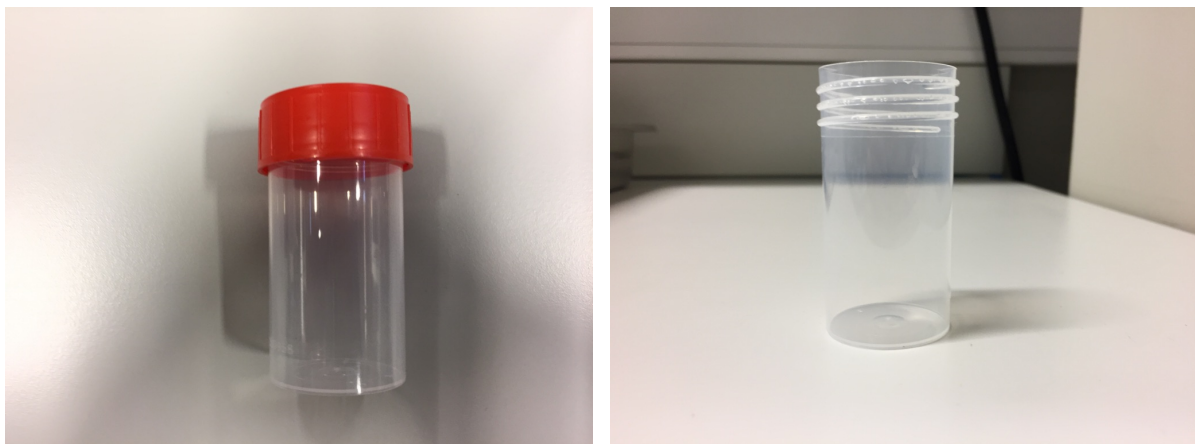
Figure 32. Cylinder mold H: 65 mm & D: 33 mm (Kjaernsmo, 2017)
