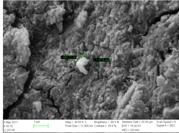
Figure 114. The smallest observed Graphene Oxide sheet. Spectrum III is located in the center of the bright object. (Kjaernsmo, 2017)
