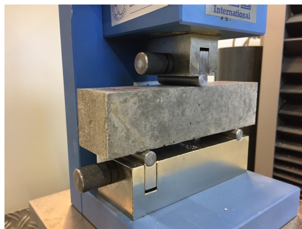
Figure 55. Flexural strength testing jig with tilting roller supports (Kjaernsmo, 2017)
