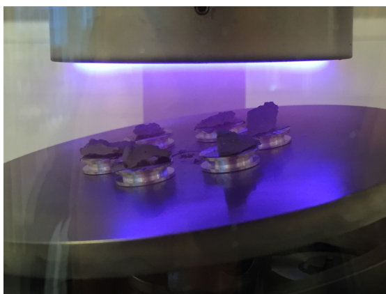
Figure 69. Small samples were taken from central parts from the fractured surface (Kjaernsmo, 2017)
