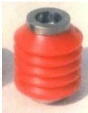
Figure 2.15: Cement dart (Portman 2004)
