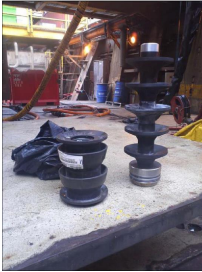
Figure 2.12: (Left) Upper and lower wiper plugs (Olsen et al. 2017); (Right) Illustration of cross-sectional barrier formed by the method (Courtesy of Statoil).
