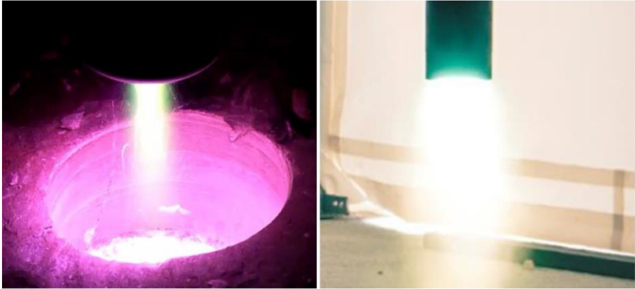
Figure 3.1: Difference in plasma shape, (Left) narrow conventional plasma flow – (Right) Electric arc area-wide plasma flow (Kocis et al. 2015).
