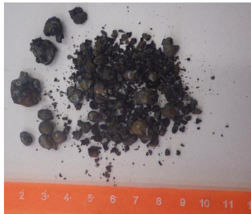
Figure 3.6c: Samples of cuttings after test done in high pressure (20MPa) brine environment. The irregularl shape large aggregates were found to be several cuttings clustered together (Kristofic et al 2016).
