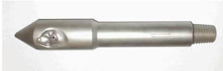
Figure 2.18: CT abrasive perforation head after completed job (Loving et al. 2005)
