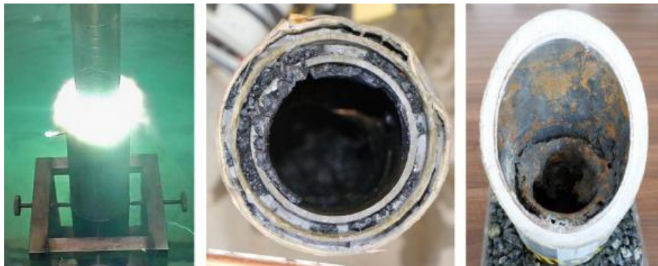
Figure 3.8: Water environment casing milling setup and results. During the same experiment it was shown that 3.5" tool was capable of milling 4.5" 5.5" and 7" casing (Gajdos et al. 2015a)
