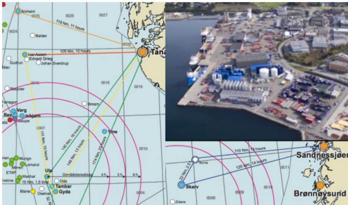
Figure 2: Left and lower right: Offshore bases and operated fields – routes, distances and sailing time (AkerBP, 2017b) Colors on sailing routes indicate designated PSV and standby-vessels. Upper right: Asco Tananger base. (Asco, 2017)
