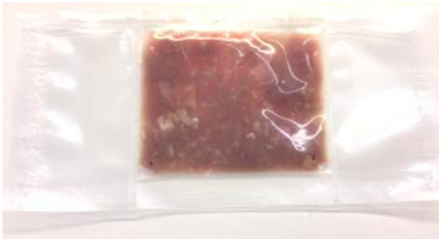
Figure 14: Bag containing 5 grams of minced meat solution rolled flat. There are empty pockets on the sides of the bag for easy attachment to the rack.
