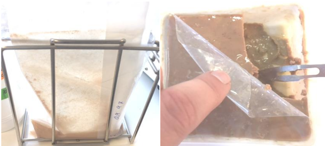
Figure 19: The liver pate samples were weighed and homogenized. Samples of 25 grams were collected in a stomacher bag and diluted 1:10 with 0.1 % Peptone water.
