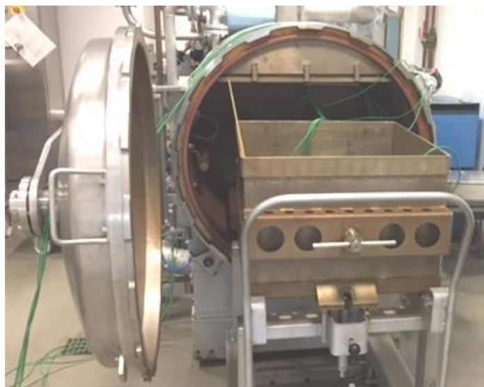
Figure 18: Steriflow autoclave used for thermal processing of the trays containing liver pate.
