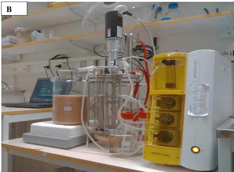
Figure 9. 5 L-capacity fermenter. A. A fed-batch recombinant protein fermentation set-up. B. Harvest of cultivated cell culture. A batch is often harvested after 16 – 20 hours of induction.
