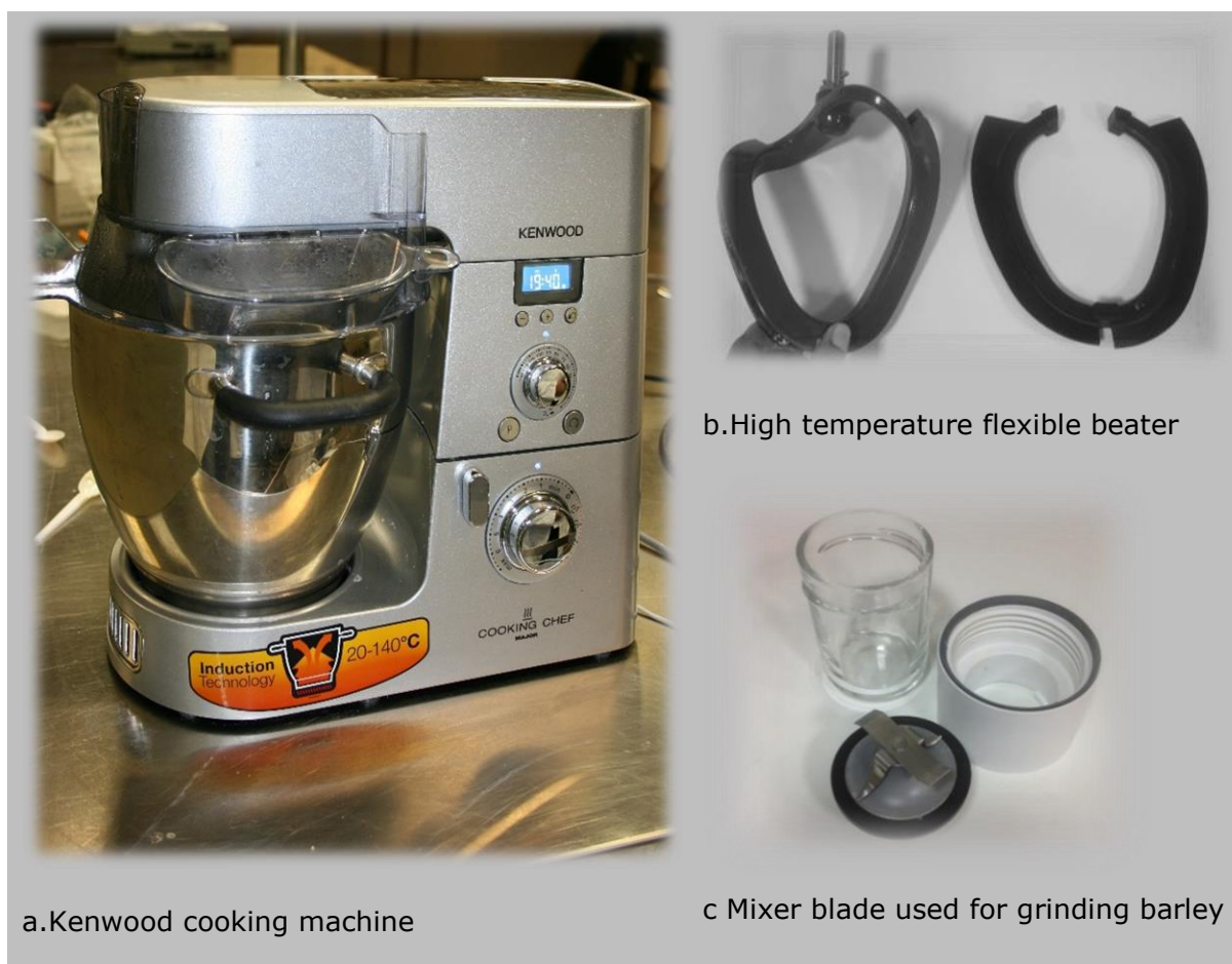
Figure 3-3: Kenwood cooking chef with the equipment used for cooking. a. Kenwood cooking chef. b. High temperature flexible beater. c. Mixer attached on top of Kenwood where the lid was removed and mixer with a blade was fixed to attachment outlet.
