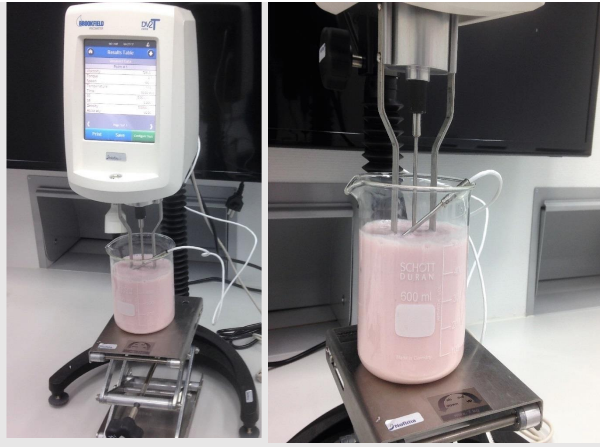
Figure 3-10: Brookfield viscometer(DV2T) extra with thermometer, spindle and guard leg placed into the sample poured in 600ml griffin beaker.
