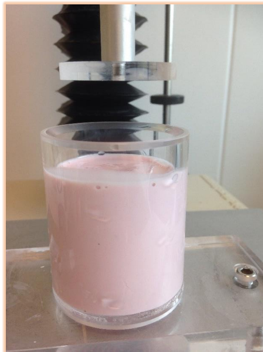
Figure 3-9: The disc plunger ready to immerse into the sample placed on the centre of fixed base.
