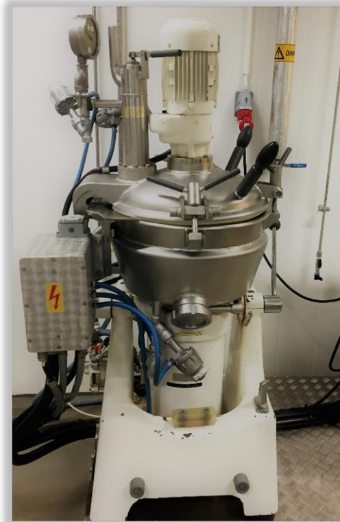
Figure 3-2: Stephan vessel from Stephan food processing machinery
