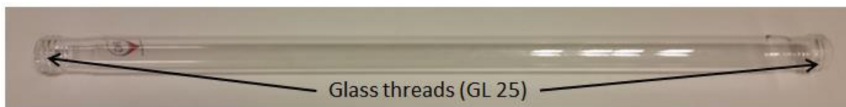
Figure 4-1 An imbibition tube with glass threads on each end side and glass filter type 2 inside the inlet tube (Haugland, 2016)
