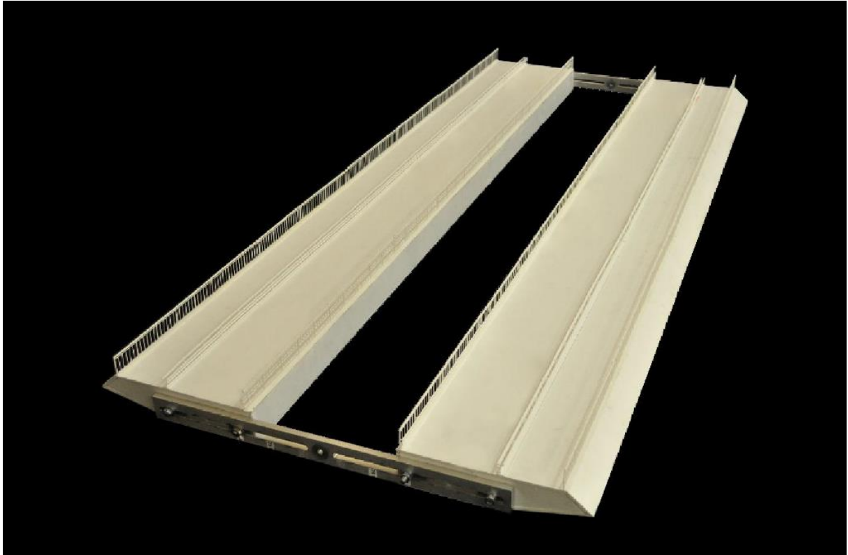
Figure 1. Section model of the Halsafjorden bridge (Hansen et al. (2016))
